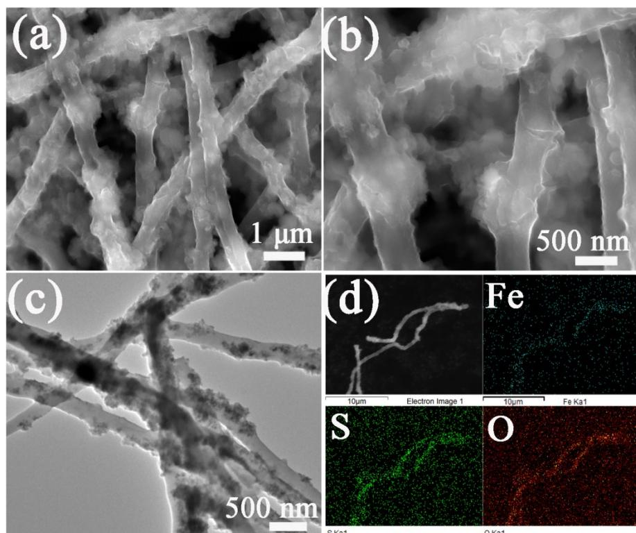
Fig. S8. Typical SEM (a, b) and TEM (c) images of  $2\text{-FeS}_2/\text{Fe}_2\text{O}_3@\text{N}$ -CNFs electrodes after 600 cycles with different magnification; (d) SEM elemental mapping images of the cycled  $2\text{-FeS}_2/\text{Fe}_2\text{O}_3@\text{N}$ -CNFs fibers.
