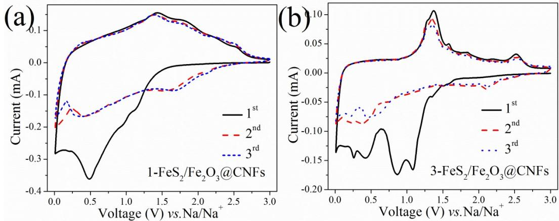
Fig. S3. (a) CV curves of 1-FeS<sub>2</sub>/Fe<sub>2</sub>O<sub>3</sub>@N-CNFs and 3-FeS<sub>2</sub>/Fe<sub>2</sub>O<sub>3</sub>@N-CNFs obtained at scan rate of 0.1 mV s<sup>-1</sup>.
