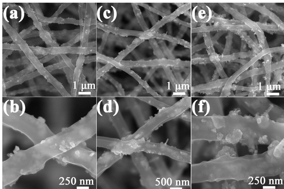
Fig. S1. SEM images of the as-obtained FeS<sub>2</sub>/Fe<sub>2</sub>O<sub>3</sub>@N-CNFs with different sulfuration time (a, b) 1-Fe<sub>2</sub>O<sub>3</sub>@N-CNFs, (c, d) 2-FeS<sub>2</sub>/Fe<sub>2</sub>O<sub>3</sub>@N-CNFs and (e, f) 3-FeS<sub>2</sub>/Fe<sub>2</sub>O<sub>3</sub>@N-CNFs.
