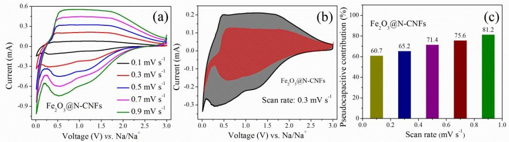
Fig. S5. (a) CV curves of  $\text{Fe}_2\text{O}_3@\text{N-CNFs}$  electrode with different scan rates; (b) the calculated capacitive current contribution from the CV curves at scan rate of  $0.3 \text{ mV s}^{-1}$ ; (c) the pseudocapacitive contribution proportion of  $\text{Fe}_2\text{O}_3@\text{N-CNFs}$  at different scan rates.
