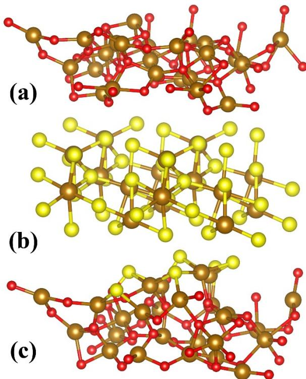
Fig. S9. Optimized geometry structures of (a)  $\text{Fe}_2\text{O}_3$ , (b)  $\text{FeS}_2$  and (c)  $\text{Fe}_2\text{O}/\text{FeS}_2$  heterostructure.
