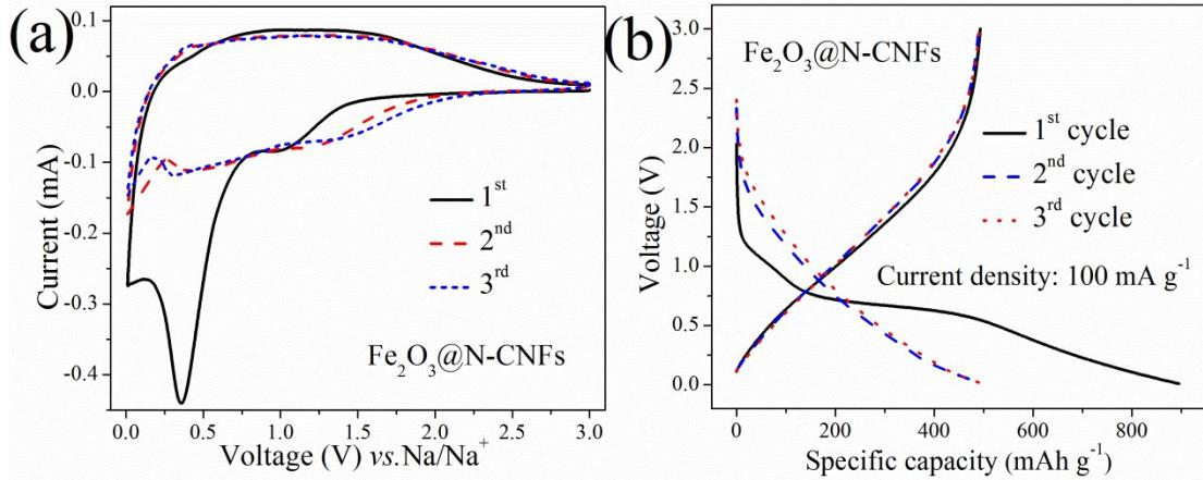
Fig. S2. (a) CV curves and (b) galvanostatic charge/discharge profiles of  $\text{Fe}_2\text{O}_3@\text{N-CNFs}$  electrode.
