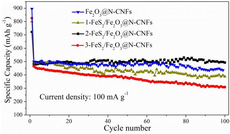
Fig. S4. Cyclic performance of the as-obtained samples in a voltage window of 0.01-3.0 V with a current density of  $100 \text{ mA g}^{-1}$ .
