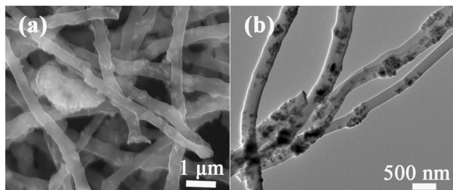
Fig. S7. SEM (a) and TEM (b) images of  $\text{Fe}_2\text{O}_3@\text{N}$ -CNFs electrode obtained after 600 cycles at current density of  $1 \text{ A g}^{-1}$ .
