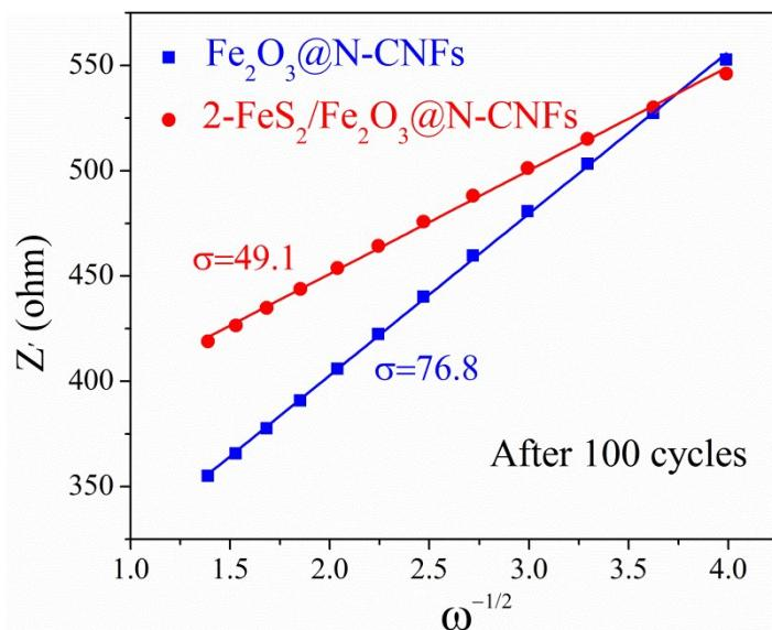
Fig. S6. Linear relationship of the real impedance against the minus square root of the frequency
