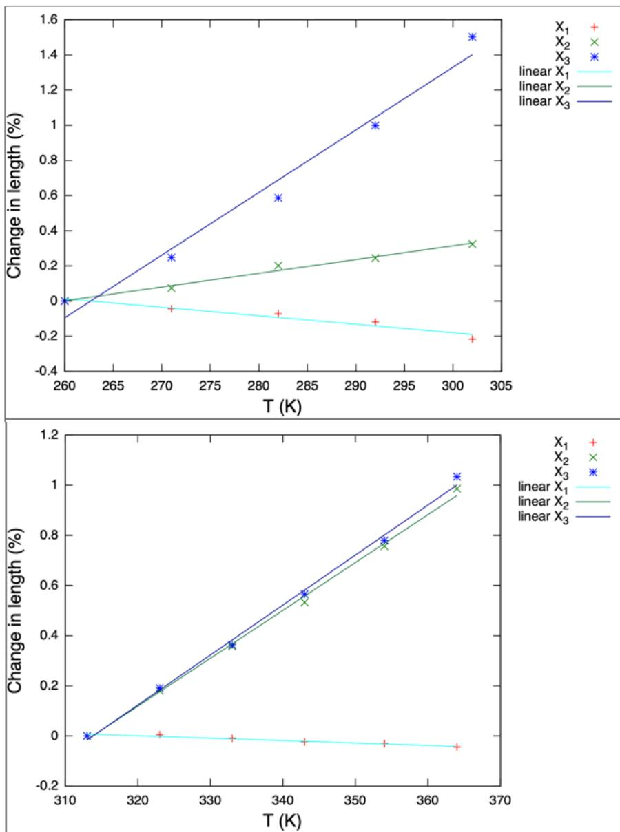
**Fig. S8.** Changes in lengths of the principal orthogonal axis of phase **III** and **II** as a function of temperature (experimental data are shown in Figure 6). Continuous lines show the linear fitting for the calculation of the thermal expansion coefficients obtained using the PASCAL program.
