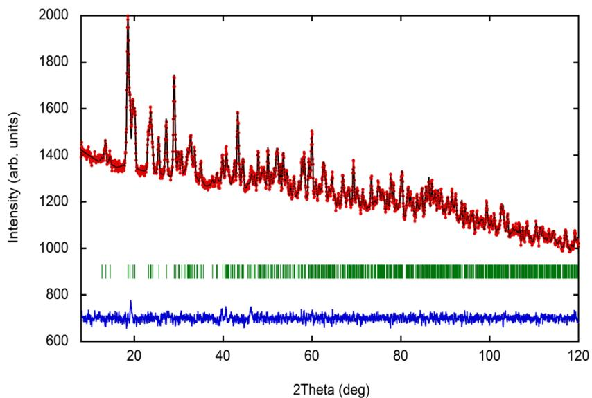
**Fig. S7:** Rietveld refinement to the D2B data at 10 K. Observed (red points) and calculated (black solid line) powder diffraction patterns for positions of the Bragg reflections are represented by green vertical bars. The observed-calculated difference patterns are depicted as a blue line.  $R_{\text{Bragg}} = 3.84$ .
