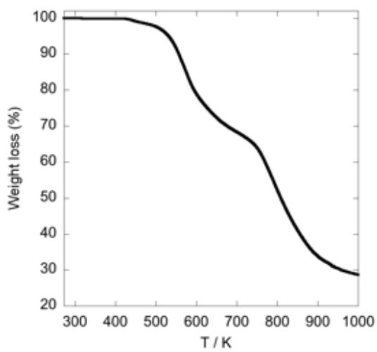
**Fig.S5.** TG curve recorded in inert atmosphere.
