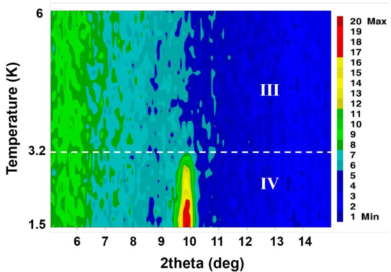
**Fig.S11.** NPD thermodiffractogram of ((R)-(-)-3-hydroxyquinuclidium)[FeCl<sub>4</sub>] acquired at D1B from 1.5 to 6 K. The temperature of the disappearance of the magnetic peak is indicated with a dashed white line.
