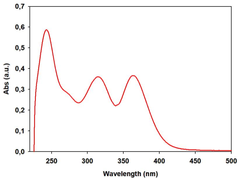
**Fig. S2.** UV-Vis spectrum of ((R)-(-)-3-hydroxyquinuclidium)[FeCl<sub>4</sub>] in CH<sub>2</sub>Cl<sub>2</sub> at 25 °C.
