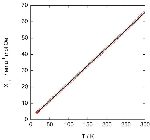
**Fig. S10.** Fit to the Curie-Weiss law (solid black line) to the magnetic susceptibility data at 1 kOe.
