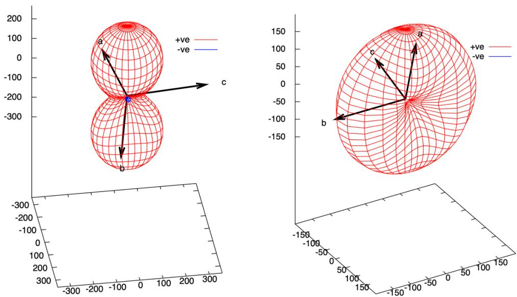
**Fig. S9.** The thermal expansion indicatrices (red positive; blue negative) of Phase **III** (left) and **II** (right) related to the crystallographic axes (black).
