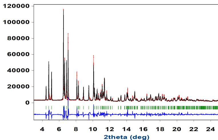
**Fig.S6:** Rietveld refinement to the SR-XRPD data at 100 K. Observed (red points) and calculated (black solid line) powder diffraction patterns for positions of the Bragg reflections are represented by green vertical bars. The observed-calculated difference patterns are depicted as a blue line.  $R_{\text{Bragg}} = 6.87$ .
