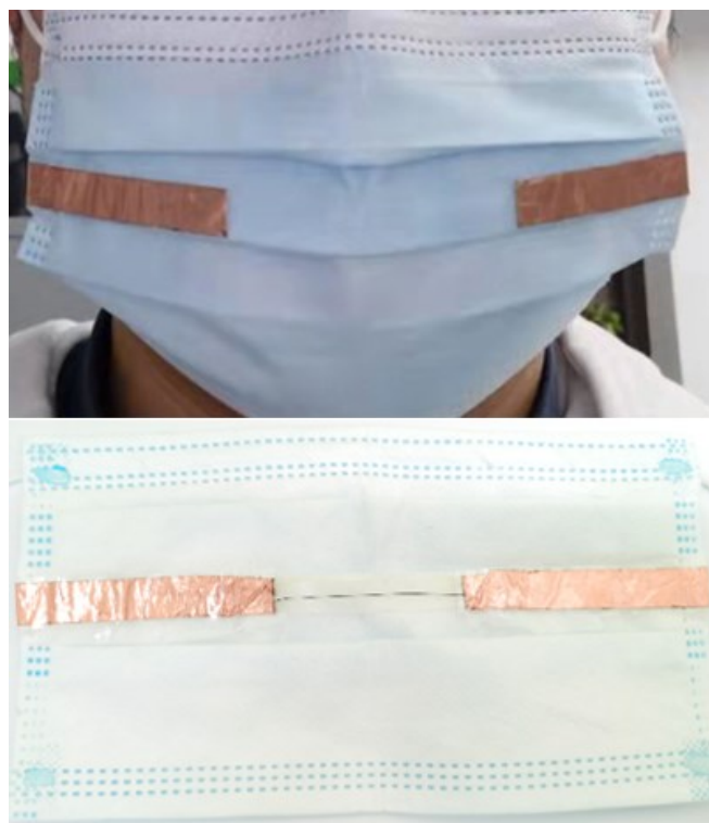
Figure S19. A respiratory monitoring sensor based on CG10 fiber; transparent insulating tape was pasted on the copper glue to avoid the interference of human body to the electrical signal.
