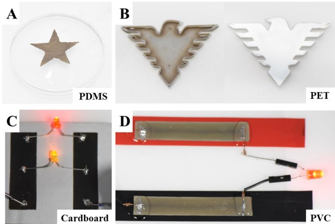
**Figure S1.** LML ink can sintered on PDMS (A), PET (B), cardboard (C), and PVC (D) to form conductive paths.
