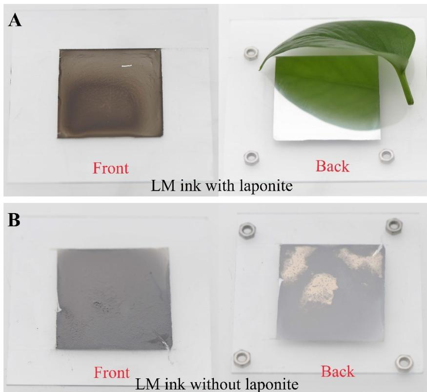
**Figure S2.** The difference between LM ink with laponite and without laponite after evaporation. The leaf is used to show the mirror-like back side.
