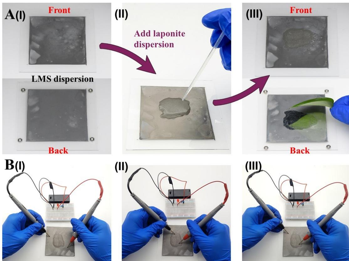
**Figure S4.** Laponite aqueous dispersion post-sintered LM nanoparticles wrapped with sodium alginate.
