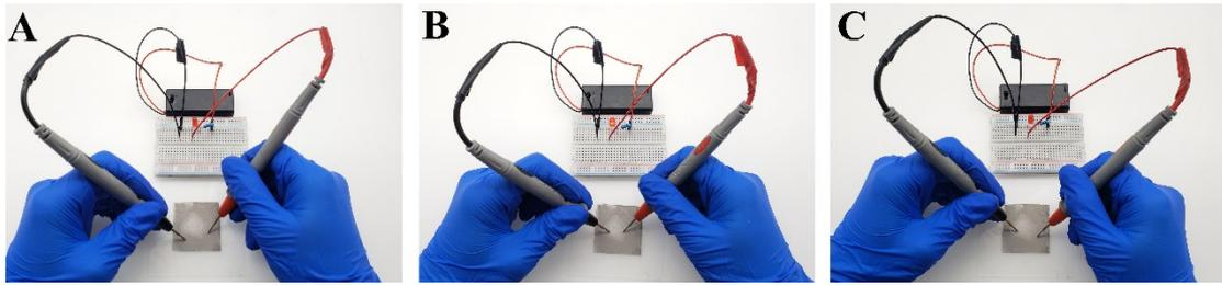
**Figure S3.** Laponite aqueous dispersion can post-sinter LM nanoparticles. The LM nanoparticles were precipitates formed after LM ink evaporating to dryness, and the LM ink was prepared by sonicating the mixture of bulk LM and water in ice-water bath for 30 minutes.
