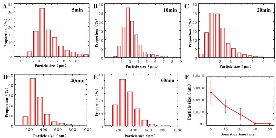
**Figure S6.** Changes of liquid metal particle size distribution with ultrasonic time, with LM concentration of 40mg/ml and laponite concentration of 1% (w/v).
