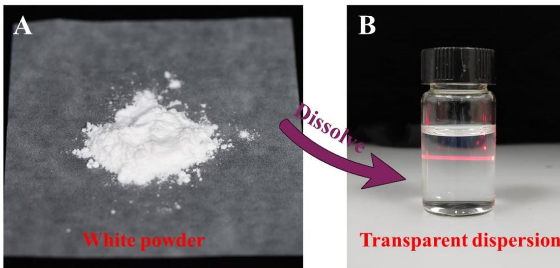
**Figure S7.** The optical images of laponite powder and laponite transparent dispersion. Laponite transparent dispersion exhibits Tyndall effect.
