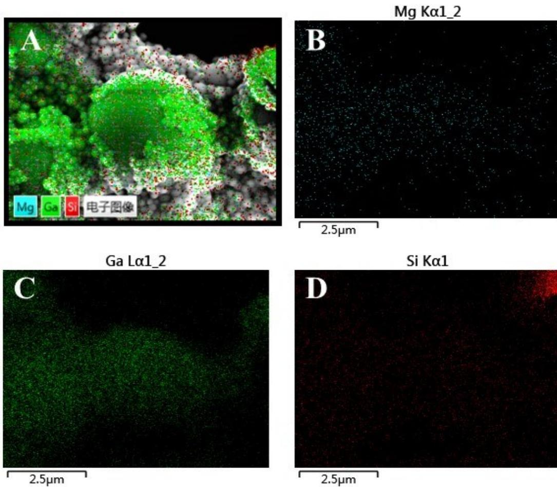
**Figure S5.** The Mg, Ga, Si elemental mapping of LM droplets.
