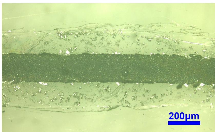
**Figure S9.** Optical microscope image of the minimum line-width prepared with LML ink.
