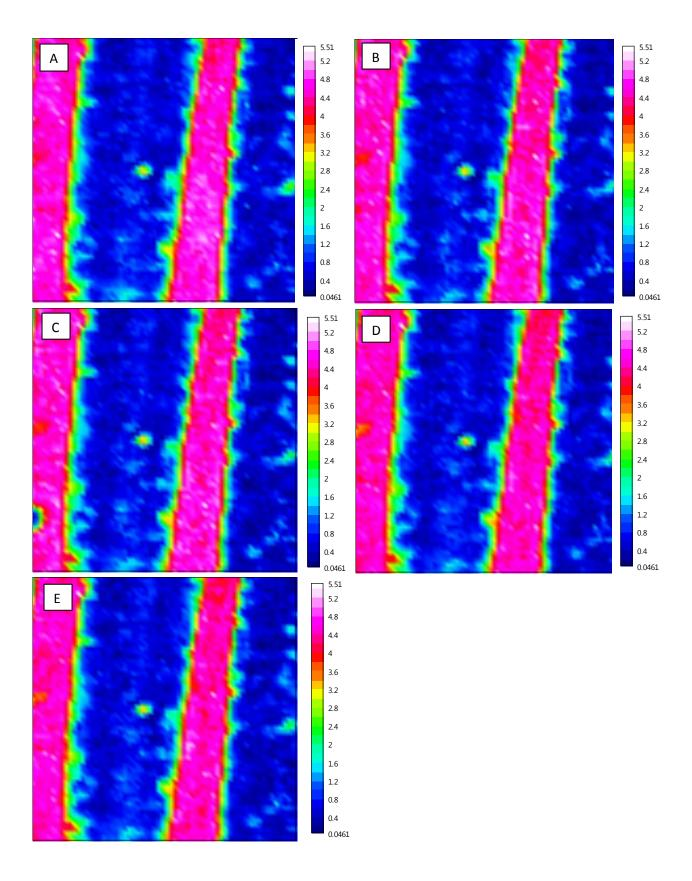
**Supplementary Figure 1.** Integrated absorbance of the amide I band showing 30 mg/ml lysozyme in channels under flow for FTC 1 (A) to 5 (E)
