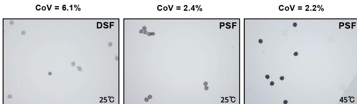
**Figure S3.** Images of color labeled DSF and PSF hydrogel microparticles after enzyme reaction in different enzyme reaction temperatures. Coefficient of variation (CoV) values of the colorimetric signal intensity in each case are represented above the images.
