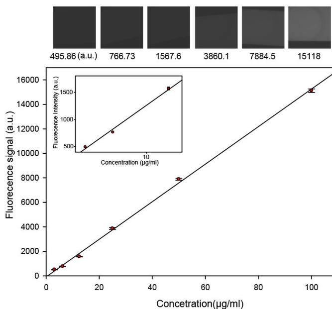
**Figure S2.** A calibration curve of streptavidin-phycoerythrin (SA-PE) solution in  $24\ \mu\text{m}$ -height channel. Each data point represents average signal of SA-PE solution.
