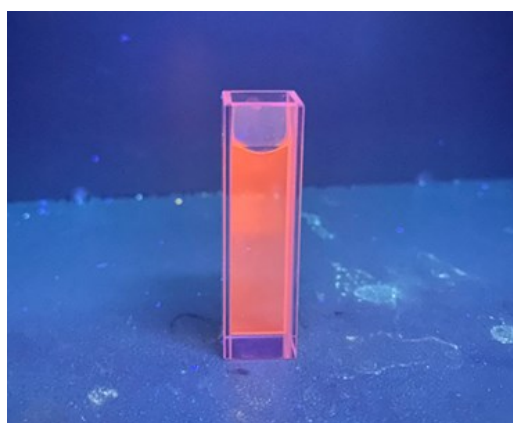
Fig. S2 Photographs of AuNCs solutions under UV light (302 nm).
