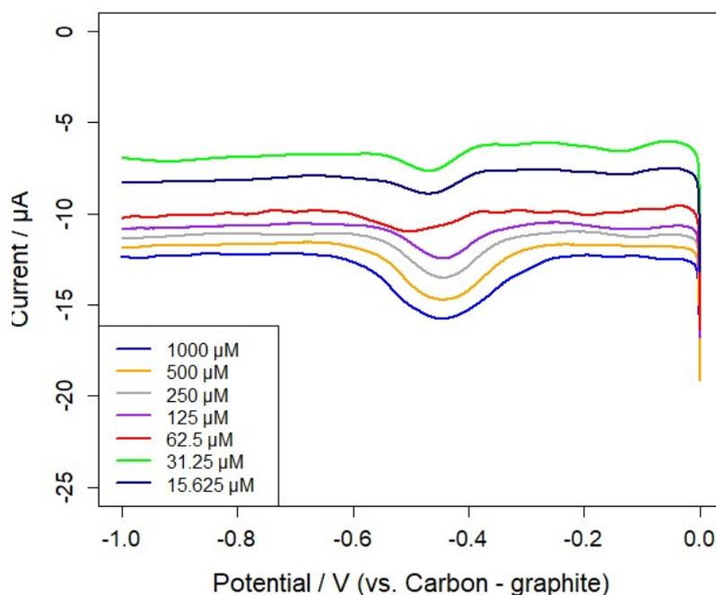
Figure S2. Differential pulse voltammogram current response versus potential for resazurin concentrations of 1000 to 15.625  $\mu\text{M}$ . using bare SPEs.
