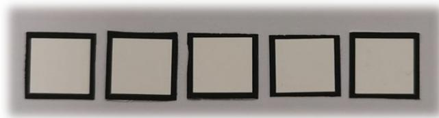
**Figure S5 Photograph of paper-based chips in nitrocellulose membrane.** The side length of the square hydrophilic area was 10 mm.
