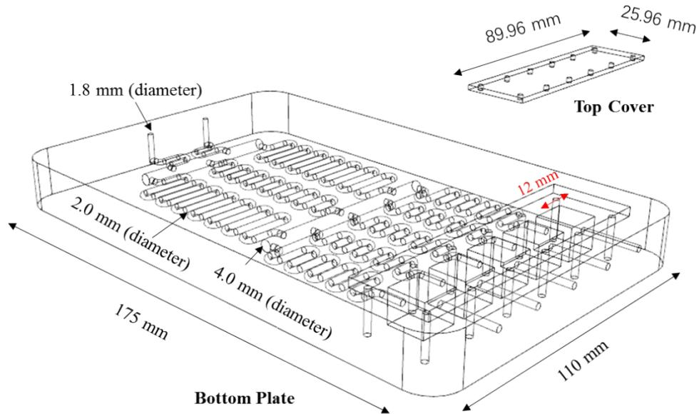
Figure S1. The outline diagram of 3D printed microfluidic chip
