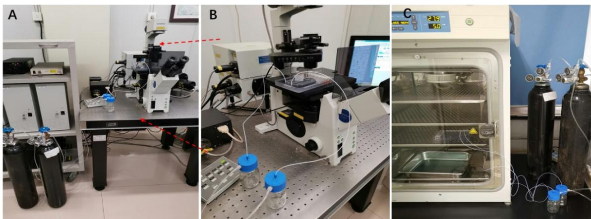
**Figure S3. The working photograph of oxygen gradients-generating chip.** (A) The working photograph of detecting oxygen concentration in the cell culture chambers with laser scanning confocal microscope. (B) is partial graph of (A). (C) The working photograph of oxygen gradients-generating chip for cell culture.
