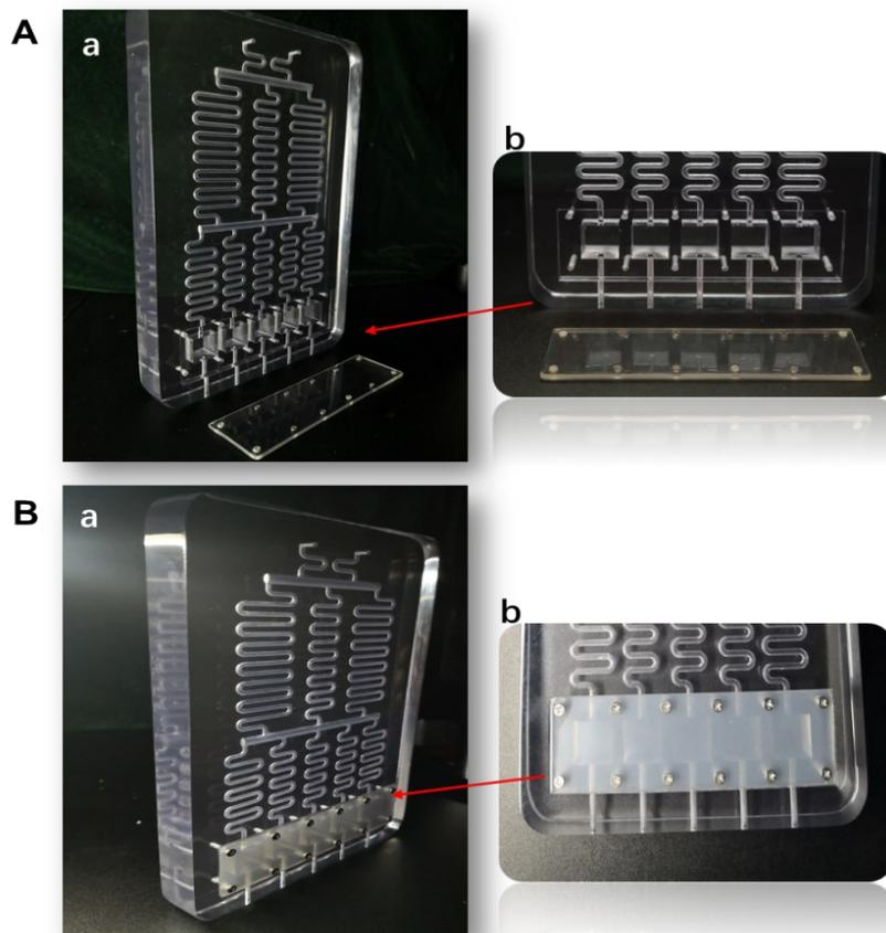
Figure S2. Pictures of 3D printed microfluidic chip. (A) The bottom plate and top cover of 3D printed microfluidic chip. (B) The two pieces of the chip and soft silicone pad were assembled with screws.
