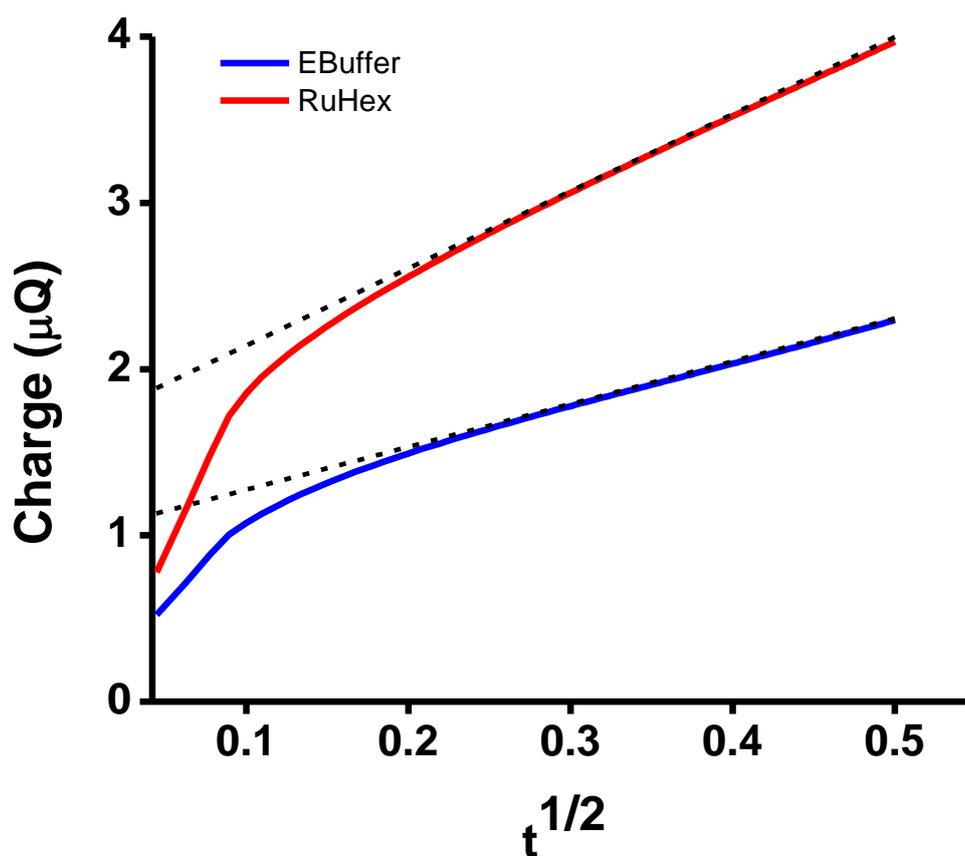
**Figure S2:** Chronocoulometric responses for screen-printed gold electrodes (SPGEs) modified with self-assembled monolayer (SAM) of thiolated capture probes in the presence of E-buffer (10 mM Tris-HCl; pH 7.0) and RuHex (50  $\mu\text{M}$  ruthenium hexamine  $[\text{Ru}(\text{NH}_3)_6]^{3+}$  solution in E-buffer).
