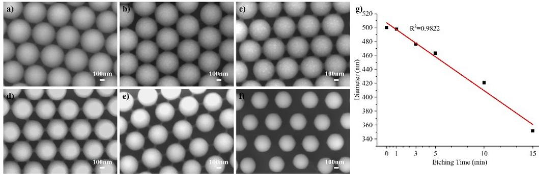
**Figure S2.** a-f) SEM images of PS at etching time of 0, 1, 3, 5, 10, 15 min, respectively, g).
