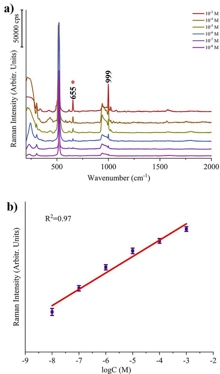
**Figure S8.** a). SERS spectra of TPhT of varying concentrations from  $10^{-3}$  to  $10^{-8}$  M by HC5-Ag substrate; b). Log-log correlation graph of the intensity at  $655 \text{ cm}^{-1}$  and TPhT concentrations. The error bar was obtained by three replicated determinations.
