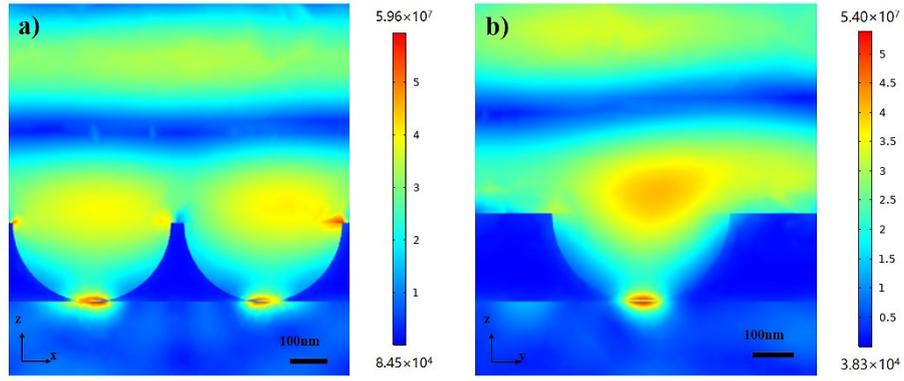
**Figure S5.** a). Electromagnetic field distribution of the substrate HC5-Ag: the x-z longitudinal section, b). Electromagnetic field distribution of the substrate HC5-Ag: the y-z longitudinal section.
