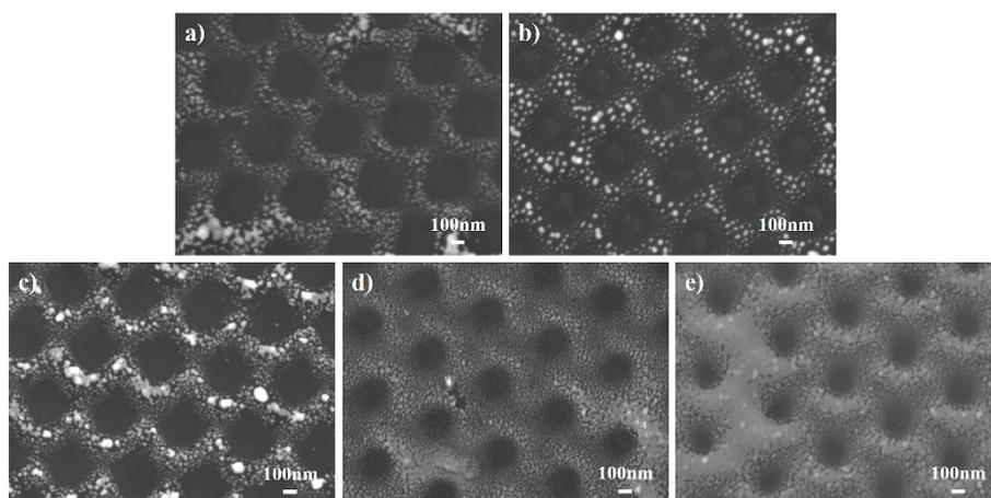
**Figure S3.** SEM images of honeycomb-like Ag arrayed structure at different etching time: a-
