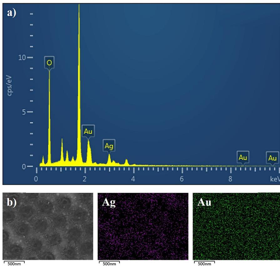
**Figure S4.** a) EDS analysis of HC5-AgAu substrates, b) EDS mapping results of HC5-AgAu substrates.
