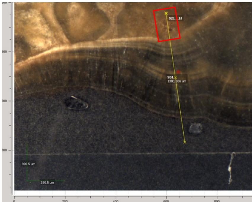
Figure 4. Image of the analyzed line from sample S32 represented in Figure 2. Highlighted in red is the region described as COM with organic matter.
