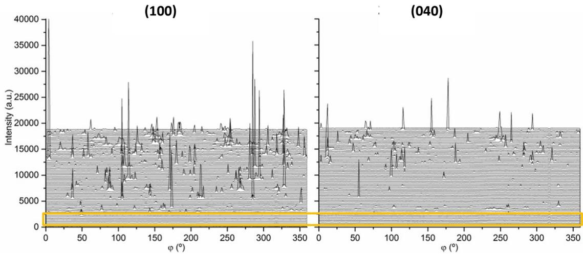
Figure 5. Representation of the azimuthal integration on the reflections (100) (Left) and (040) (Right) of a kidney classified as a transformed COD (S31). Orange square (bottom) mark the resin where the Stone is embedded.
