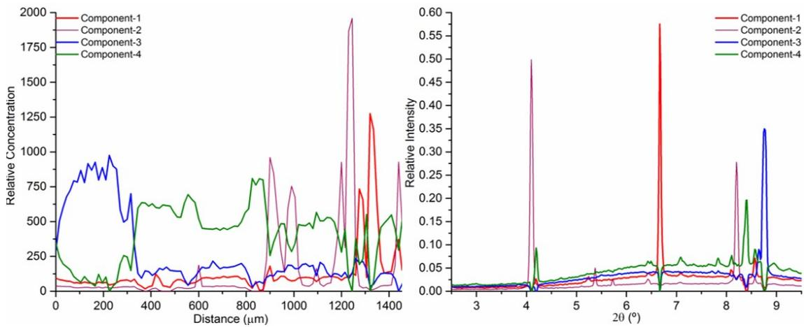
**Figure 7.** Example of MCR analysis of the diffractogram from a Correlated transformation from the superficial deposit of sample S24. In the left panel, the evolution of the four components along the diffraction analysis (from the surface to the inside of the stone) is represented, while on the right panel the simulated patterns for each component is shown.
