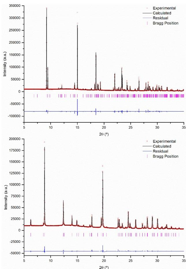
Figure 1. XRD pattern of the synthesized COM (top) and COD (bottom) after the profile matching
