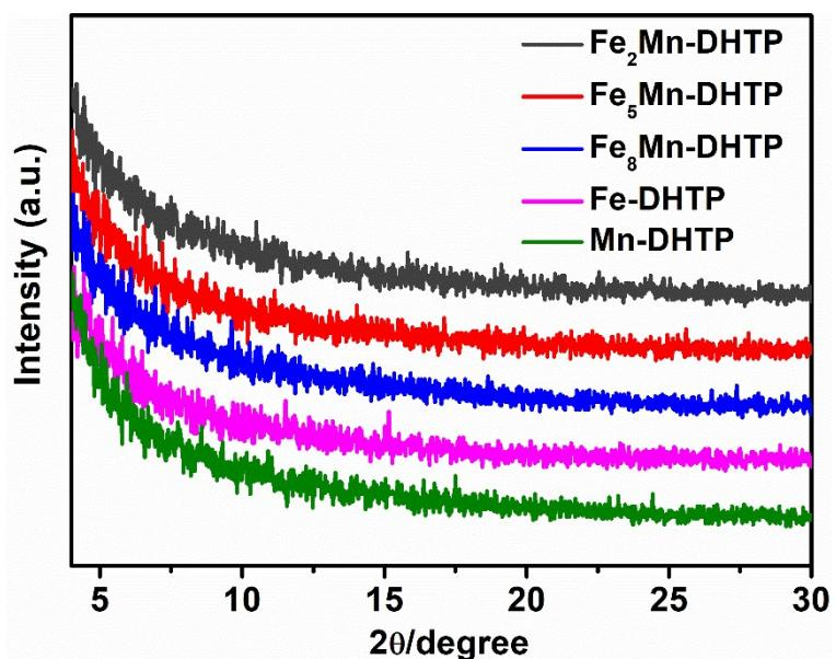
**Fig. S2** PXRD patterns of Fe<sub>2</sub>Mn-DHTP, Fe<sub>5</sub>Mn-DHTP, Fe<sub>8</sub>Mn-DHTP, Fe-DHTP and Mn-DHTP.
