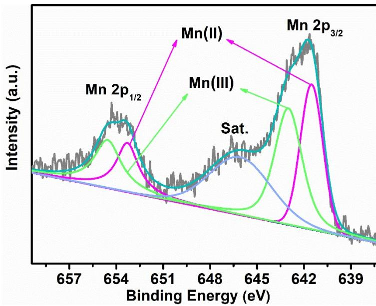
**Fig. S5** High resolution XPS spectra of Mn 2p of Fe<sub>5</sub>Mn-DHTP.
