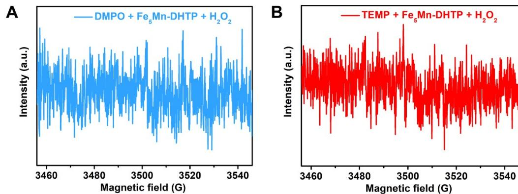
**Fig. S6** The EPR spectra of (a) Fe<sub>5</sub>Mn-DHTP methanol suspension and (b) Fe<sub>5</sub>Mn-DHTP aqueous suspension.
