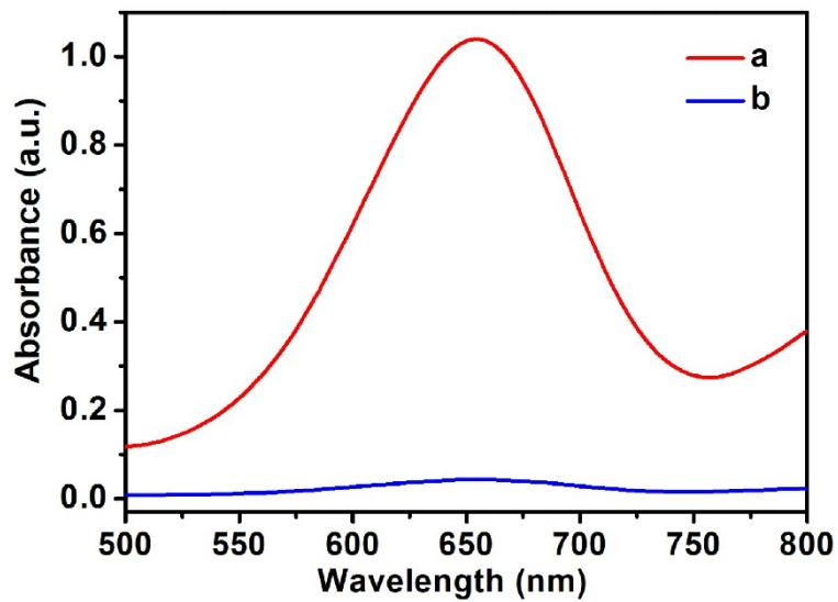
**Fig. S7** UV-vis spectra of  $\text{H}_2\text{O}_2 + \text{TMB}$  solutions in presence of (a) fresh  $\text{Fe}_5\text{Mn-DHTP}$  and (b) recycled  $\text{Fe}_5\text{Mn-DHTP}$  after treated with Cys.
