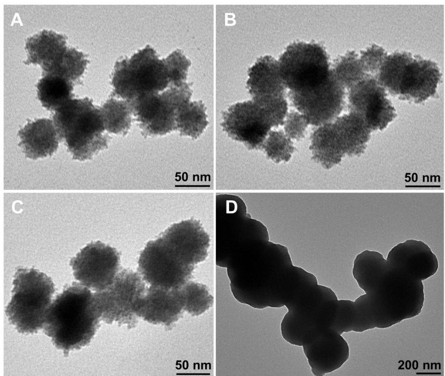
**Fig. S1** TEM images of (A) Fe-DHTP, (B) Fe<sub>2</sub>Mn-DHTP, (C) Fe<sub>8</sub>Mn-DHTP and (D) Mn-DHTP.
