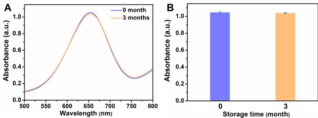
**Fig. S4** The storage stability of Fe<sub>5</sub>Mn-DHTP.
