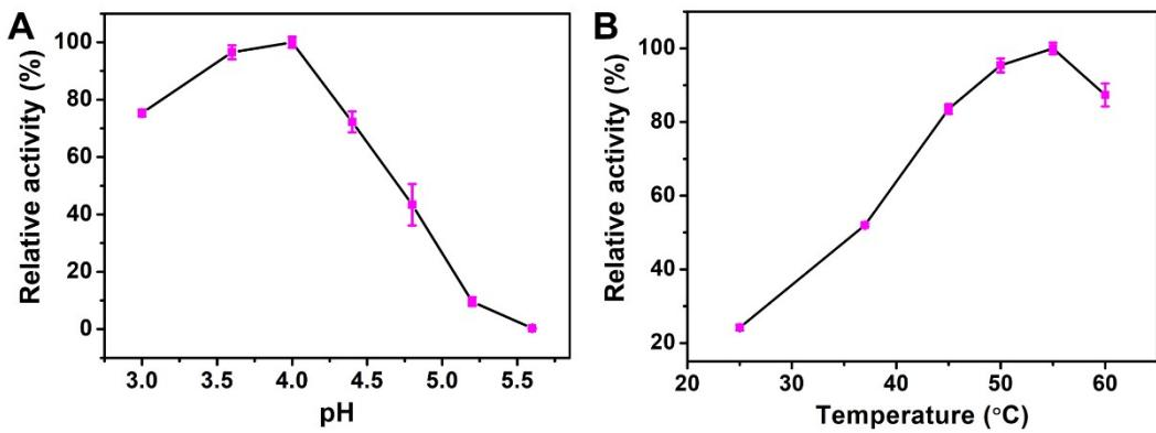
**Fig. S3** Relative activity of Fe<sub>5</sub>Mn-DHTP as a function of (A) buffer pH and (B) temperature.
