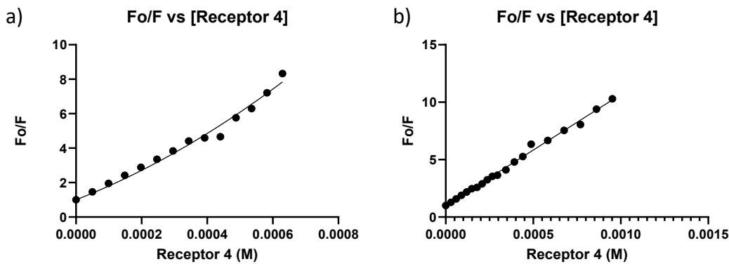
**Figure S12.** a) Stern-Volmer plot of first 14 titration points to reveal positive curvature, b) full stern-volmer plot of extended titration points.
