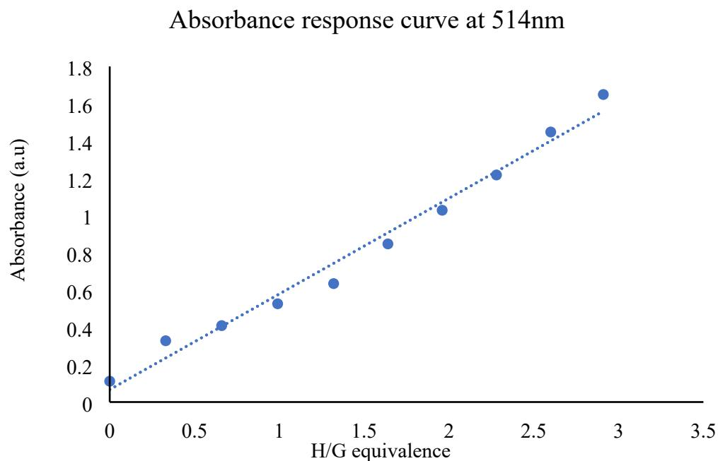
**Figure S19.** Linear response plot of absorbance at 514nm vs equivalence of host/guest in 10% HSA samples.
