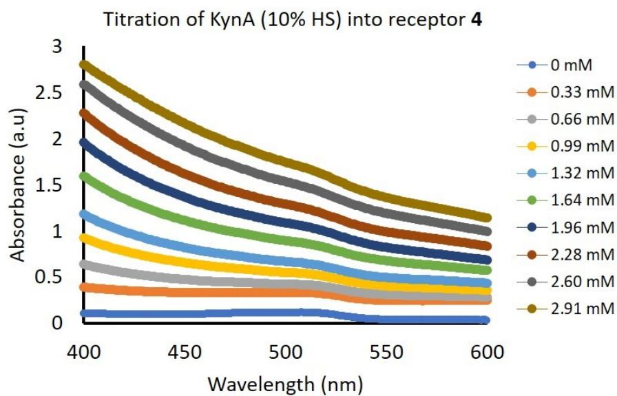
**Figure S18.** UV-Vis titration of increasing concentration of 60mM KynA in 50:40:10 DMSO/H<sub>2</sub>O/Human Serum, into a solution of 3mM receptor **4** in 90:10 H<sub>2</sub>O/DMSO system.
