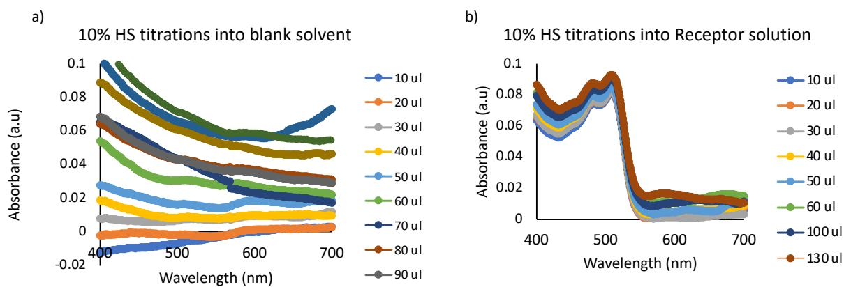
**Figure S20.** a) UV-Vis titration of increasing concentration of 50:40:10 DMSO/H<sub>2</sub>O/Human Serum (HS), into a blank solution of 90:10 H<sub>2</sub>O/DMSO system. b) UV-Vis titration of increasing concentration of 50:40:10 DMSO/H<sub>2</sub>O/Human Serum, into a solution of 3mM receptor **4** in 90:10 H<sub>2</sub>O/DMSO system in the absence of KynA.
