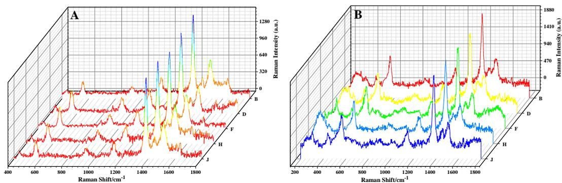
**SI\_Figure 3.** Reproducibility of SERS spectra of (A) TTD ( $1.0 \times 10^{-5}$  M) and (B) TTD with of  $\text{Hg}^{2+}$  ( $1.0 \times 10^{-7}$  M). The RSD for TTD and  $\text{Hg}^{2+}$  are 3.41% and 1.35%, respectively.
