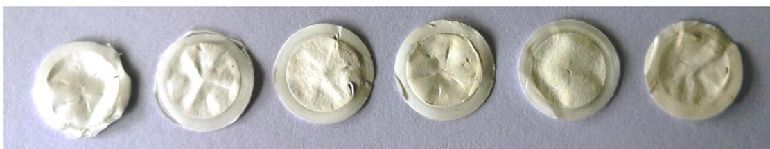
**SI\_Figure 1.** Optical images of Ag-decorated polymer films with different soaking time from 0 to 5 h (from left to right are 0, 1, 2, 3, 4, and 5 h).
