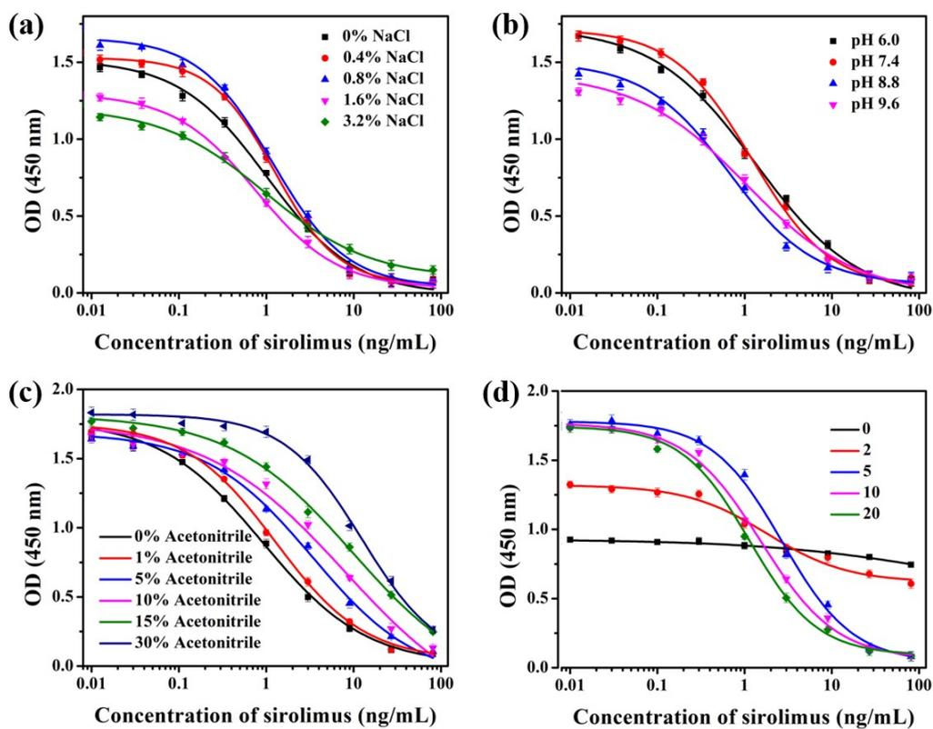
Fig. S1 (a) The optimization of ic-ELISA with different content of NaCl in PBS buffer; (b) the optimization of ic-ELISA with different pH values in PBS buffer; (c) the optimization of ic-ELISA with different content of acetonitrile in PBS buffer; (d) the standard curve for sirolimus detection in human whole blood samples with different dilution ratios.
