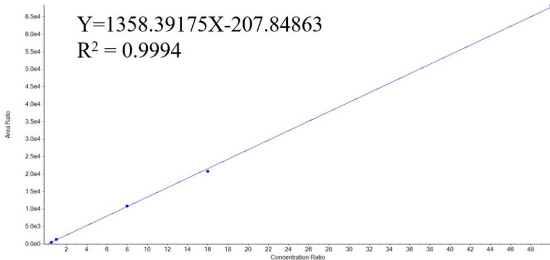
Fig. S3 The calibration curve of sirolimus in acetonitrile by LC-MS/MS.
