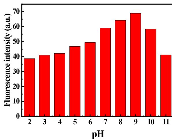
**Figure S7.** Fluorescence spectra of Cys-Au NCs under different pH conditions. Experimental condition: Cysteine (1.5 mM), NaOH (6 mM), Ag<sup>+</sup> (30.0 μM) and HAuCl<sub>4</sub> (1 mM); reaction time, 3 h; reaction temperature: 90 °C, PB buffer solution (6.0-8.0), BR buffer solution (2.0-11.0).
