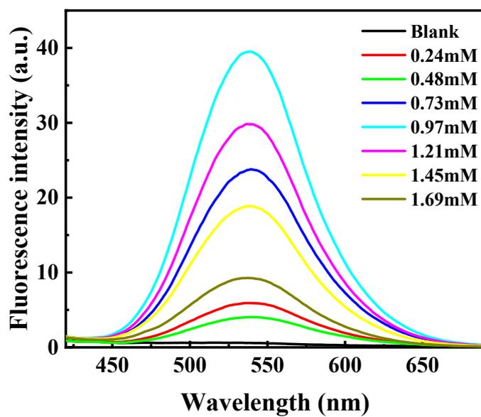
**Figure S6.** Fluorescence spectra of Cys-Au NCs-Ag<sup>+</sup> with different concentration of Cys-Au NCs in the range from 0.24 mM to 1.69 mM. Experimental condition: Cys-Au NCs (1.5 mM, represented by the concentration of HAuCl<sub>4</sub>), Cysteine (1.5 mM), NaOH (6 mM), Ag<sup>+</sup> (30.0 μM) and HAuCl<sub>4</sub> (1 mM); reaction time, 3 h; reaction temperature: 90 °C.
