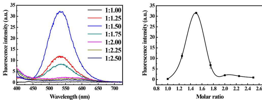
**Figure S3.** Fluorescence spectra (A) and intensity (B) of Ag<sup>+</sup> enhanced Cys-Au NCs synthesized under different molar ratio of H<sub>2</sub>AuCl<sub>4</sub> and cysteine. Experimental condition: cysteine (1.5 mM), NaOH (6 mM), Ag<sup>+</sup> (30.0 μM) and H<sub>2</sub>AuCl<sub>4</sub> (1.0 mM); reaction time, 3 h; reaction temperature, 90 °C.
