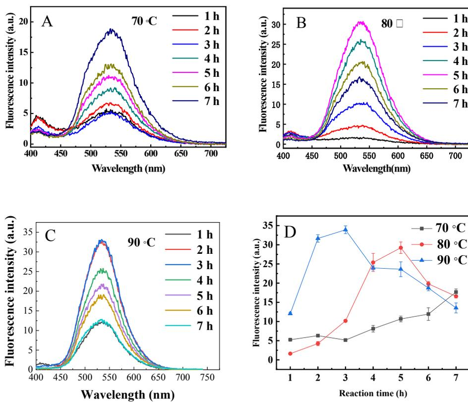
**Figure S5.** Fluorescence spectra of Ag<sup>+</sup> enhanced Cys-Au NCs synthesized under different temperature and different reaction time: 70 °C (A), 80 °C (B), 90 °C (C). Effect of temperature on generation of luminescent Cys-Au NCs (D). Experimental condition: cysteine (1.5 mM), NaOH (6 mM), Ag<sup>+</sup> (30.0 μM) and HAuCl<sub>4</sub> (1 mM); reaction time, 3 h; reaction temperature: 70, 80, 90 °C.
