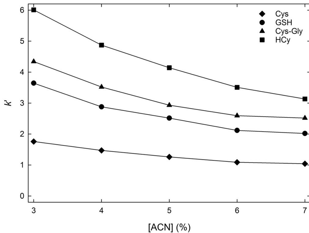
Figure S6. The observed changes in the retention factors,  $k'$ , for the amino thiols when changing the concentration of ACN from 3% to 7% in the chromatographic solvent.
