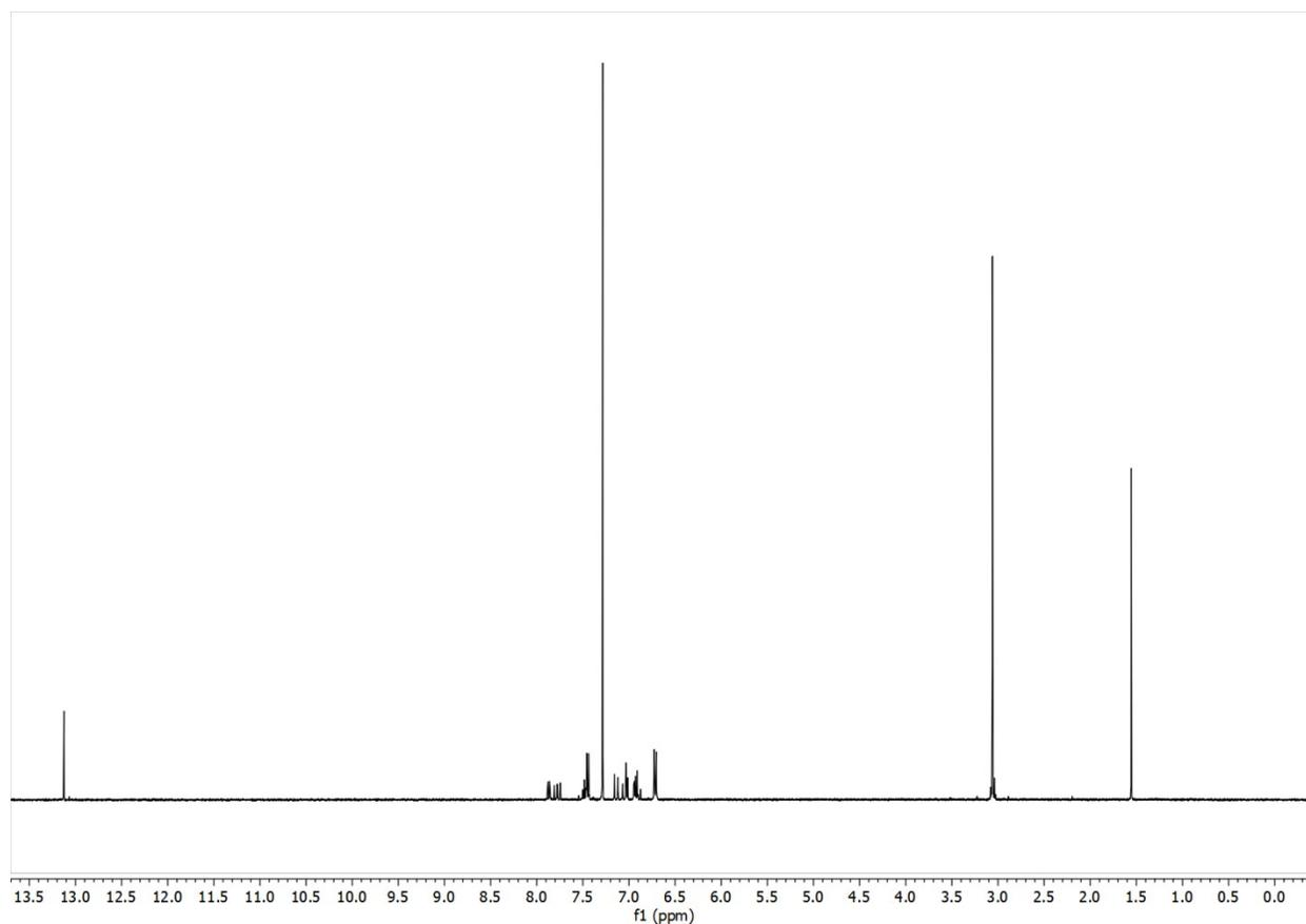
SI Figure 1.  $^1\text{H}$  NMR spectrum of compound 1 in  $\text{CDCl}_3$ .
