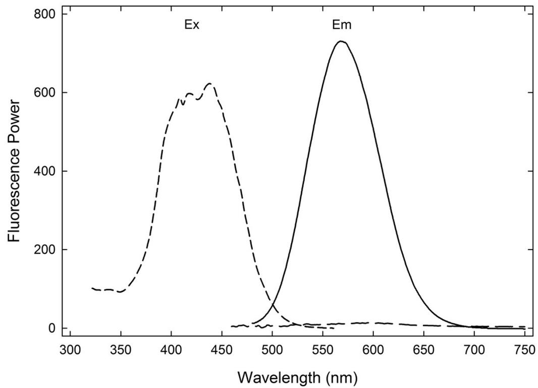
**Figure S4.** Excitation (Ex, short dash line) and emission (Em, solid line) spectra of cpd 2, and the emission spectrum of probe 3 (long dash line).
