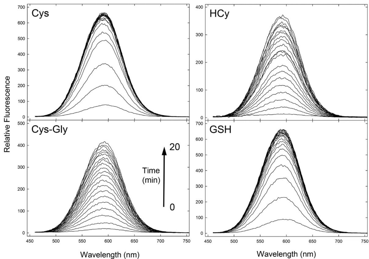
**Figure S5. Reaction progress of 35  $\mu$ M amino thiols and 40  $\mu$ M probe 3 monitored by the fluorescence of the produced cpd 2 (ex. 420 nm) over 20 minutes of reaction time.**
