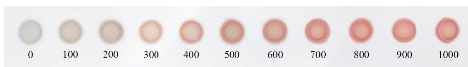
Fig. S5 A spot test platform spotted with increasing concentrations of GSH in the range 0-1000 \mu\text{g mL}^{-1} (Spot test platform – TLC, concentration of PHNZ – 1200 \mu\text{g mL}^{-1} , volume of PHNZ and GSH – 5 \mu\text{L} ).
