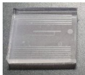
Fig. S4 Microfluidic channel made of PDMS.
