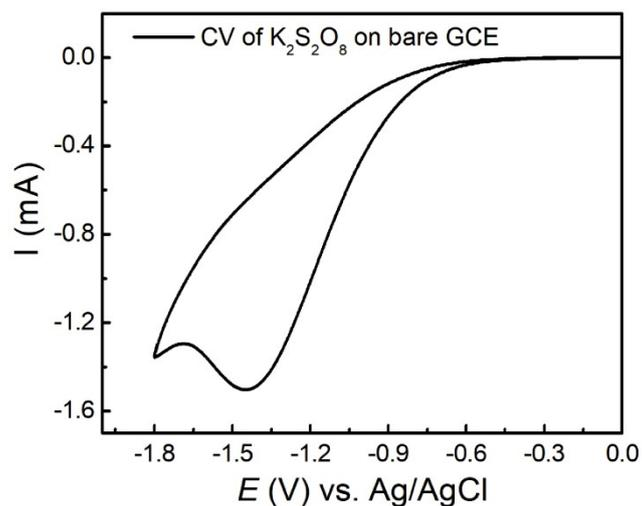
**Fig. S1** The CV of bare GCE in 0.1 M PBS solution (pH 7.4) with 0.1 M  $K_2S_2O_8$ . The scan rate was at 0.1 V/s.
