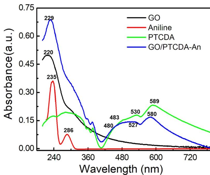
**Fig. S2** The UV-vis absorption spectroscopy of GO(black line), aniline(red line), PTCDA (green line) and GO/PTCDA-An(blue line).
