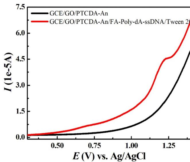
**Fig. S3** LSV of GCE/GO/PTCDA-An and GCE/GO/PTCDA-An/FA-Poly-dA-ssDNA/Tween 20 in 0.1 M PBS(pH 7.40).
