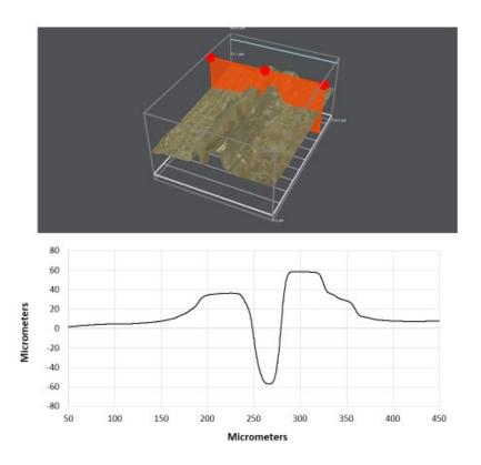
Figure S1 (top). 3D image of score topography in CN swipes. Field-of-view 450  $\mu$ m x 716  $\mu$ m. Image is a 3D optical reconstruction consisting of 46 images taken with 5  $\mu$ m vertical spacing. Figure S1(bottom). Line scan through indicated region on image showing topography of score cut.
