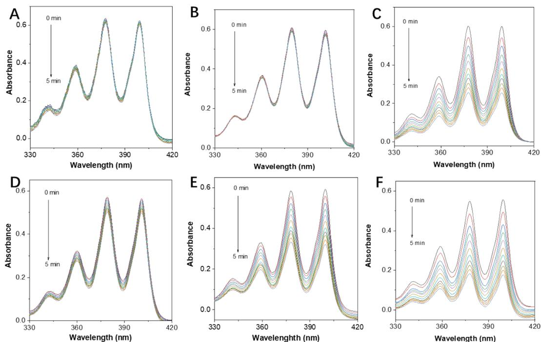
**Figure S11.** (A) UV spectra of ABDA under white light irradiation in water PBS solution. (B) UV spectra of ABDA in the presence of Rose bengal under white light irradiation in water PBS solution. UV spectra of ABDA in the presence of TPE-BEP assembly white light irradiation at different pH PBS solutions: (C) pH = 7.4, (D) pH = 6.0, (E) pH = 5.0, (F) pH = 4.0. [TPE-BEP] = [Rose bengal] = 10  $\mu\text{M}$ , [ABDA] = 50  $\mu\text{M}$ .
