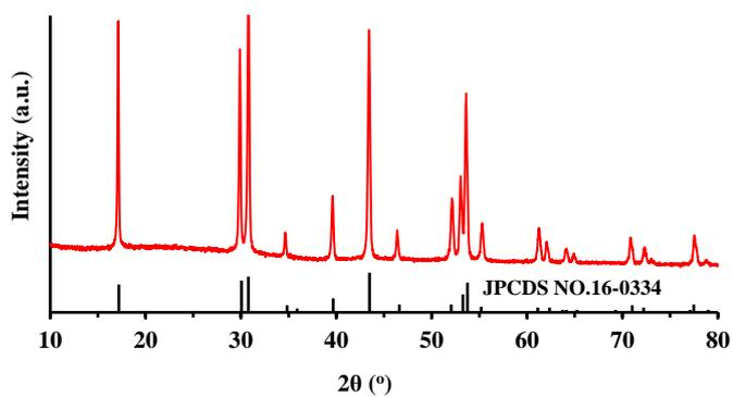
**Figure S6.** XRD patterns of UCNPs and JCPDS card.
