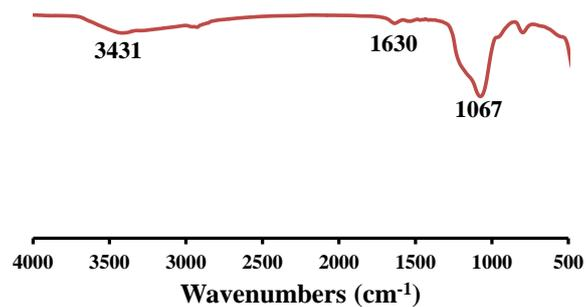
**Figure S7.** FT-IR spectra of ASUCNPs.
