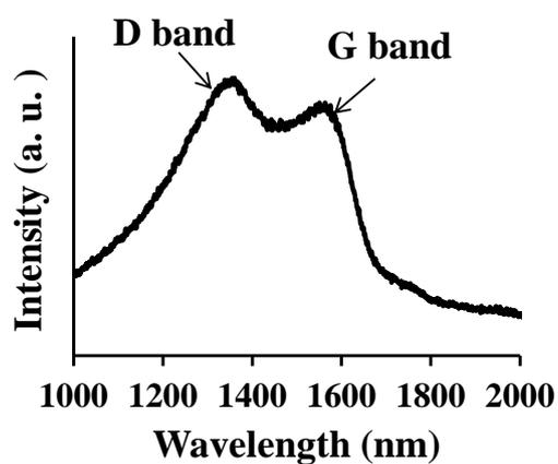
**Figure S2.** Raman spectrum of N, S co-doped GQDs GQDs.
