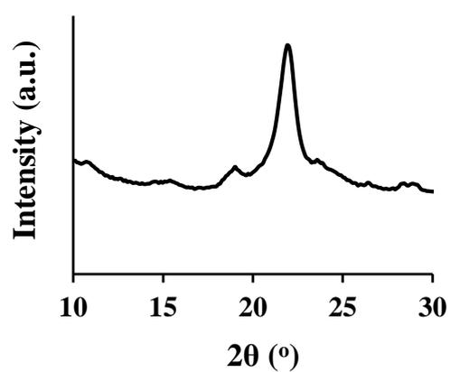
**Figure S1.** XRD pattern of N, S co-doped GQDs.
