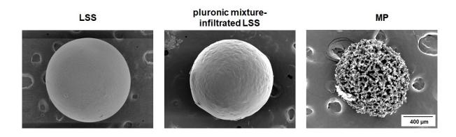
**Fig. S1** SEM photographs showing the gross appearance of LSS particle, pluronic mixture-infiltrated LSS particle, and MP particle.
