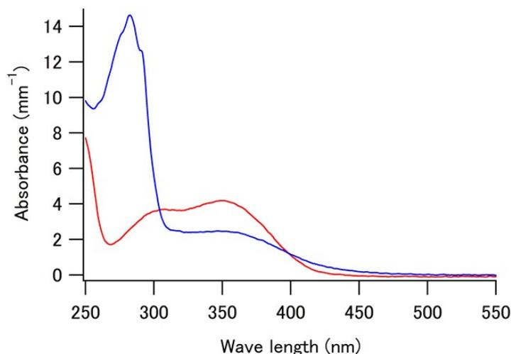
**Fig. S3** UV/vis absorbance spectra of the **PB-4armPEG** solution (red line) and the photodegraded product from the **PB-4armPEG**-avidin hydrogel (blue line).
