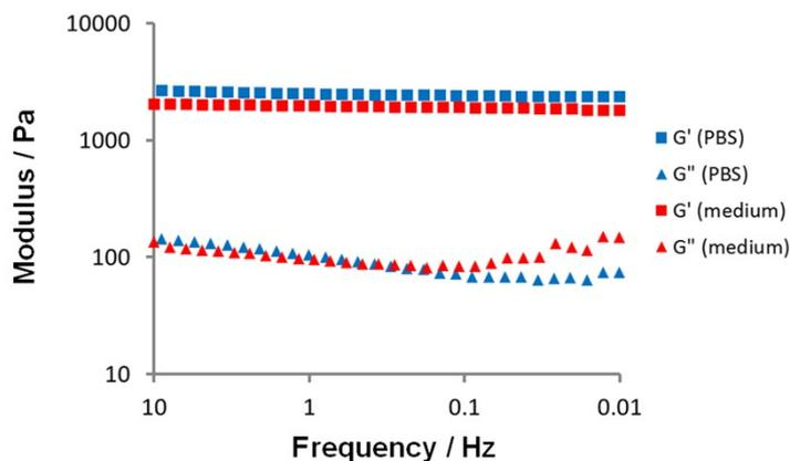
**Fig. S4** Dynamic viscoelasticity measurement of photodegradable PEG-avidin hybrid hydrogels ( $G'$ : the storage modulus (square),  $G''$ : the loss modulus (triangle)). **PB-4armPEG** and avidin were dissolved in PBS (blue) and the culture medium (red).
