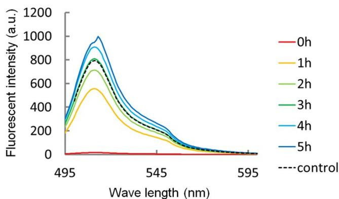
**Fig. S2** Fluorescence of EGFP released from the PEG-avidin hybrid hydrogel after incubation for various periods. The fluorescent spectra of the PBS solution on the EGFP-including hydrogel were measured after incubation for 0 (red), 1 (orange), 2 (light green), 3 (green), 4 (light blue) and 5 hours (blue). Simultaneously, that of the EGFP solution without both the macromonomer and avidin was measured as a control.
