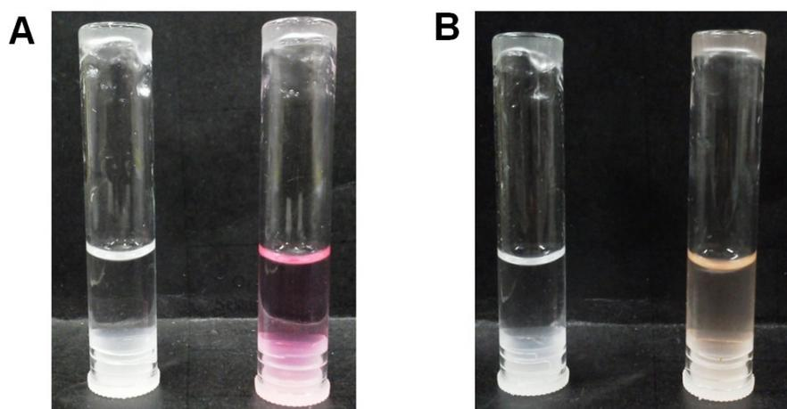
**Fig. S1** Photograph of the PEG-avidin hybrid hydrogel overlaid with solutions in the inversion test. The **B-4armPEG**-avidin hydrogel was overlaid with (*left*) PBS and (*right*) the culture medium, respectively. The photographs were taken (A) before and (B) after incubation at room temperature for 4 hours.
