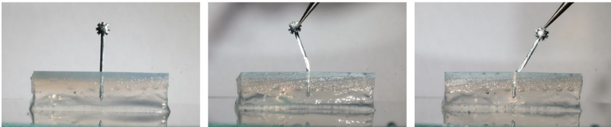
Figure S9. Optical images of a mechanically transformative needle inserted into a skin phantom (1% agarose gel) at the stiff state (left) and manipulated at the soft states (middle and right). The skin phantom is maintained at \sim 40 °C on a hot plate. The needle has been thoroughly frozen before the implantation. The implanted fraction of the needle is switched into the soft state with negligible transfer of mechanical stress to the skin phantom under external manipulations.
