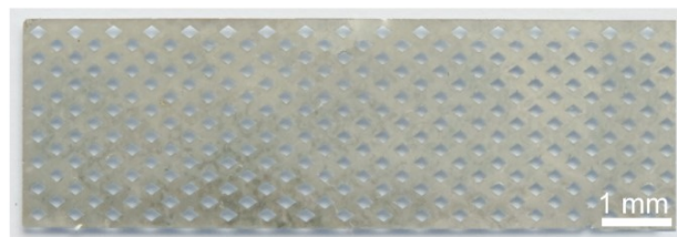
Figure S5. Optical image of a mechanically transformative mesh.
