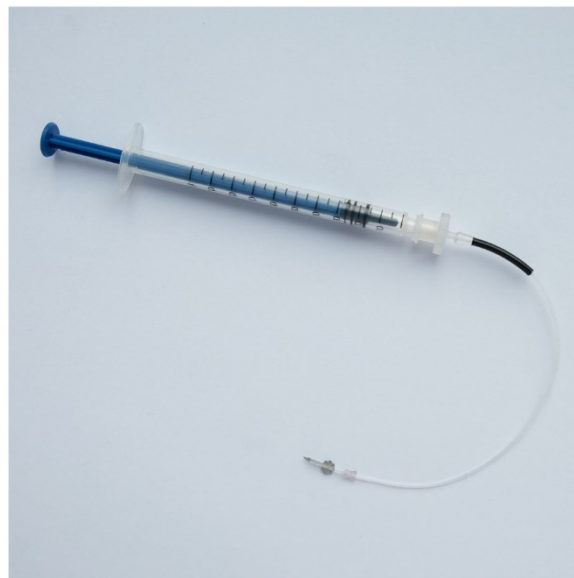
Figure S2. Optical image of a syringe barrel and indwelling needle assembly.
