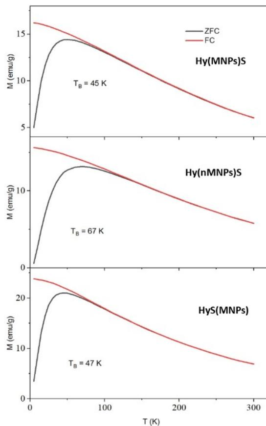
**Figure S4.** ZFC-FC curves of the samples at 100 Oe.
