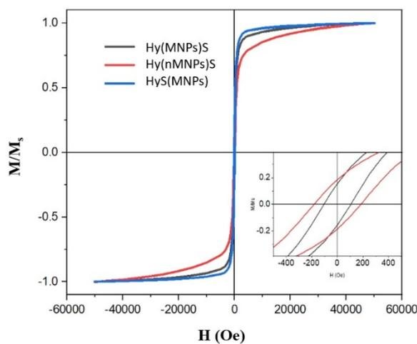
**Figure S5.** Normalized hysteresis loops at 5 K of the three samples. The inset shows a zoom at low field of samples Hy(MNPs)S and Hy(nMNPs)S
