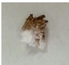
**Figure S3.** Image representing the third preparation condition in which the hybrid composite was previously prepared and subsequently soaked in a solution containing the naked nanoparticles (nMNPs). In this case the resulting scaffold was visibly inhomogeneous due to precipitation of nMNPs during drying.
