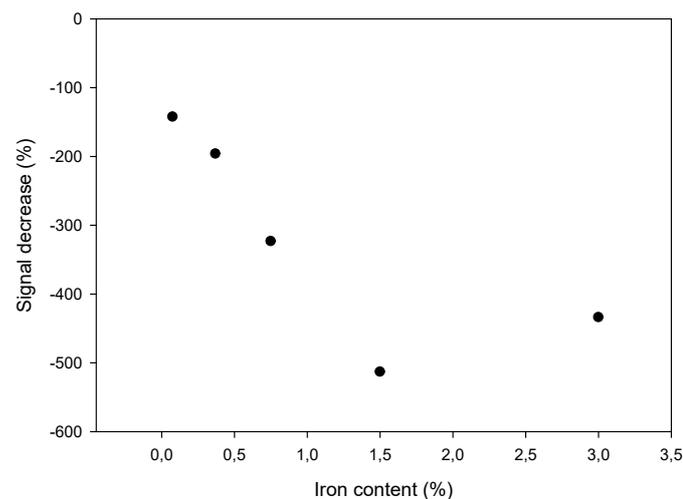
**Figure S8.** Decrease of the signal intensity (as expressed as the ratio between the signal of the magnetic matrix and the signal of the unlabelled scaffold) for the Hy(MNPs) scaffolds regarding to their iron content.
