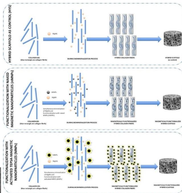
**Scheme S1.** Schematic illustration of a hypothesized mechanism about magnetic functionalization dependent on the presence of i) an activated shell (yellow ring) linking on the collagen surface (MNPs) or ii) naked nanoparticles (black core) being entrapped into collagen fibers during self-assembling of fibers (nMNPs).
