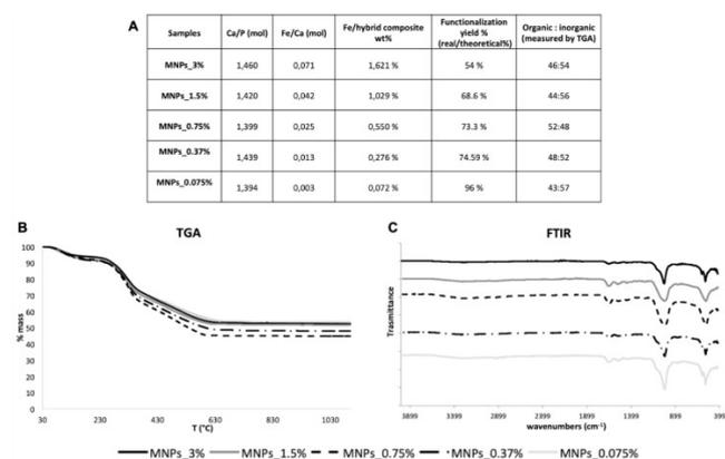
**Figure S6.** A) Chemical composition of the MNPs\_3%; MNPs\_1.5%; MNPs\_0.75%; MNPs\_0.37%; MNPs\_0.075% obtained from ICP analysis; B) Thermal decomposition profile (TG) of the MNPs\_3%; MNPs\_1.5%; MNPs\_0.75%; MNPs\_0.37%; MNPs\_0.075%, the weight loss in % of mass is used to determine the organic/inorganic ratio of the different samples; C) FTIR spectra of the MNPs\_3%; MNPs\_1.5%; MNPs\_0.75%; MNPs\_0.37%; MNPs\_0.075%.
