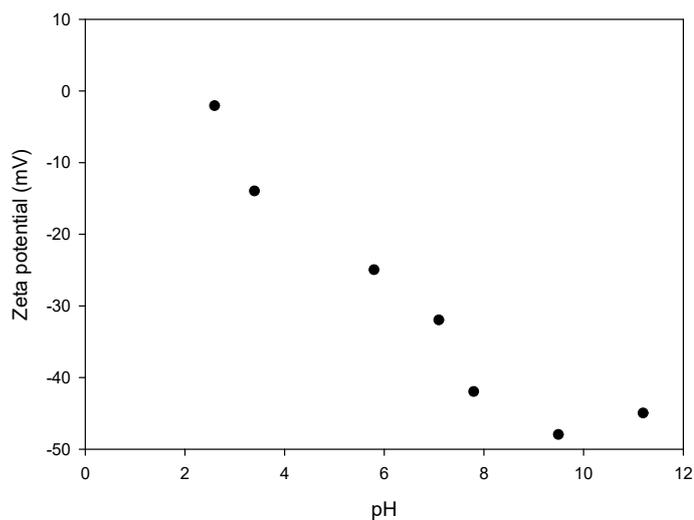
**Figure S2.**  $\zeta$ -Potential measurements vs pH of TEPSA-coated nanoparticles.
