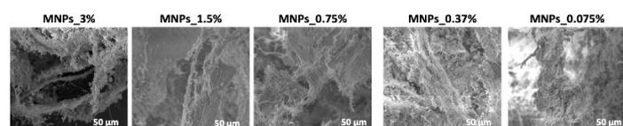
**Figure S7.** Scanning electron microscopy images of composites labeled with different amounts of MNPs (MNPs\_3%; MNPs\_1.5%; MNPs\_0.75%; MNPs\_0.37%; MNPs\_0.075%).
