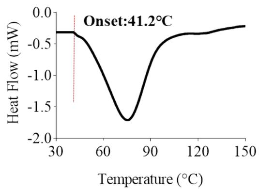
**Fig. S3** DSC curve of mPEG-PDMATC copolymer with the onset melting temperature at 41.2 °C.
