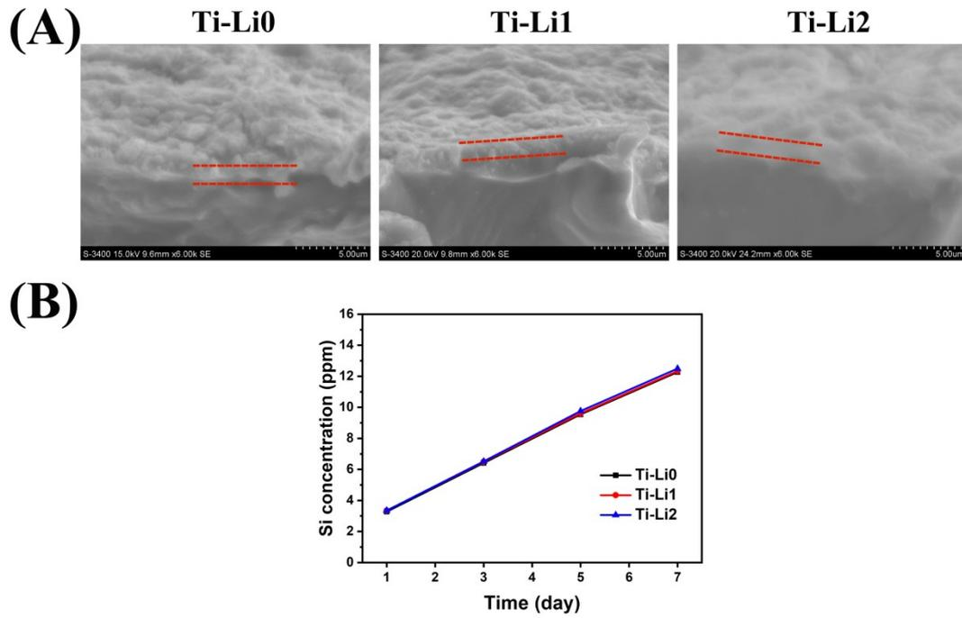
**Figure S1.** Cross-section images of PEO-coated samples (A); Cumulative release of Si ions from the PEO-coated samples incubated in deionized water for 7 days (B).
