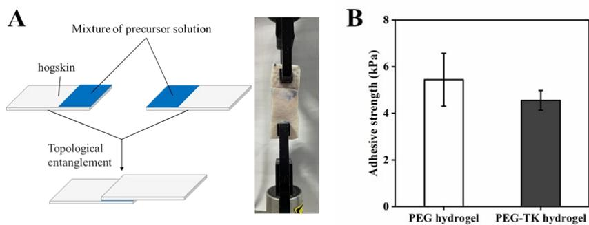
**Figure S10.** (A) Schematic presentation of the lap shear test. (B) Adhesive strength of different hydrogels on porcine skin.
