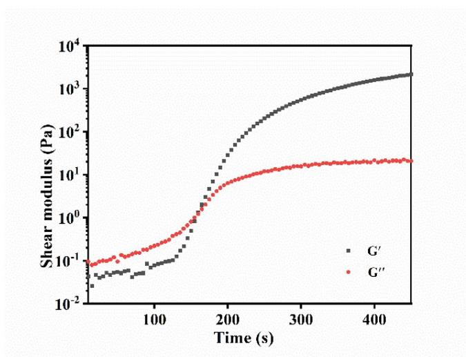
**Figure S9.** Rheological properties of the gelation process of the PEG hydrogel.
