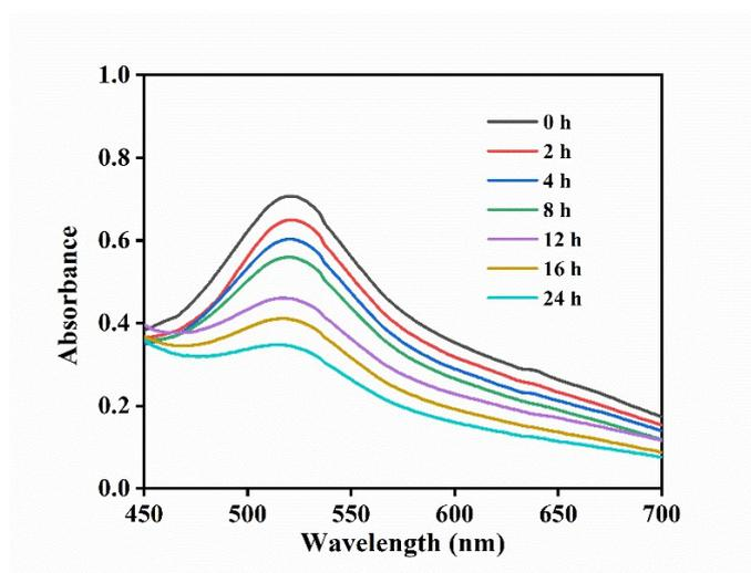
**Figure S11.** UV-vis spectra of DPPH/4-arm-PEG-TK-Nb solution within 24 h.
