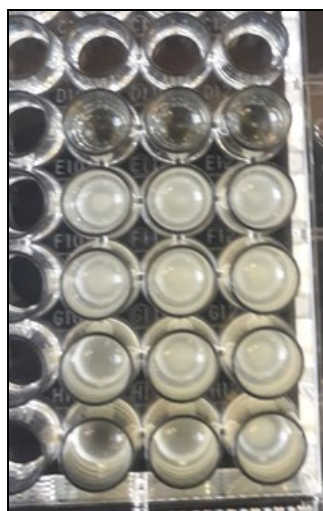
Figure S4. MIC assay performed on S. aureus in 96-well plates under different Al 2 O 3 -NPs-30 concentrations. (The red square indicates MIC value)
