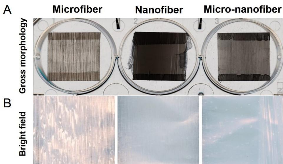
**Fig. S1** Representative gross (A) and optical (B) images of aligned microfibers, nanofibers, and micro-nanofibers.
