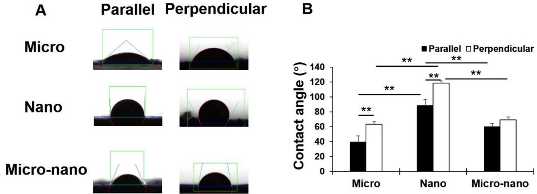
**Fig. S3** (A) Water contact angle photographs of the aligned micro-, nano-, and micro-nano porous PLLA fiber membranes taken in the directions parallel and perpendicular to the fiber axis with a video microscope. (B) Histogram shows the water contact angle data measured with the different fiber samples,  $n = 6$ . Data shown from representative sample and presented as mean  $\pm$  SD,  $**p < 0.01$ . One-way analysis of variance (ANOVA).
