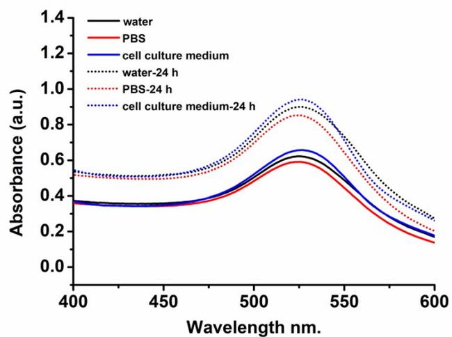
**Fig. S2** Normalized UV-vis absorption spectra of the nanoflare tracer in water, PBS and cell culture medium, respectively.
