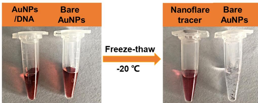
**Fig. S1** Photographs of AuNPs before and after a freeze-thaw cycle. While bare AuNPs were aggregated, adding the oligonucleotide complementary sequences (DNA1, 3  $\mu\text{L}$ , 100  $\mu\text{M}$ ) and the dye-labeled recognition sequences (DNA2-FAM, 3  $\mu\text{L}$ , 100  $\mu\text{M}$ ) protected the AuNPs from aggregation
