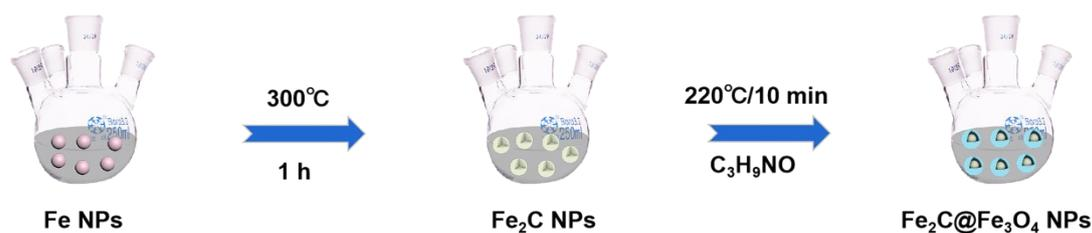
**Figure S1.** The synthesis schematic of Fe<sub>2</sub>C@Fe<sub>3</sub>O<sub>4</sub> NPs.
