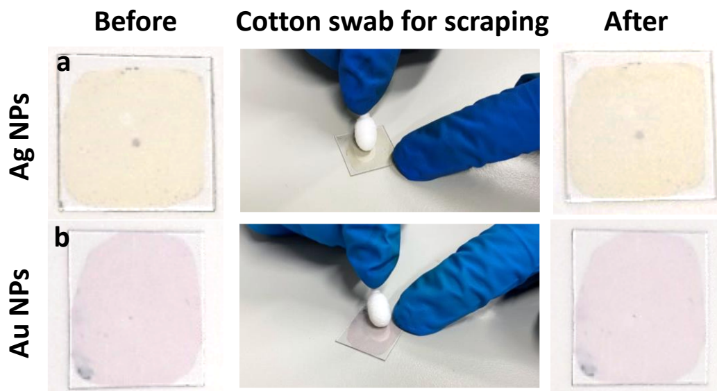
Figure S20. The images of PC substrates prepared with 10-nm (a) AgNPs and (b) AuNPs before and after being scraped with a cotton swab 20 times.
