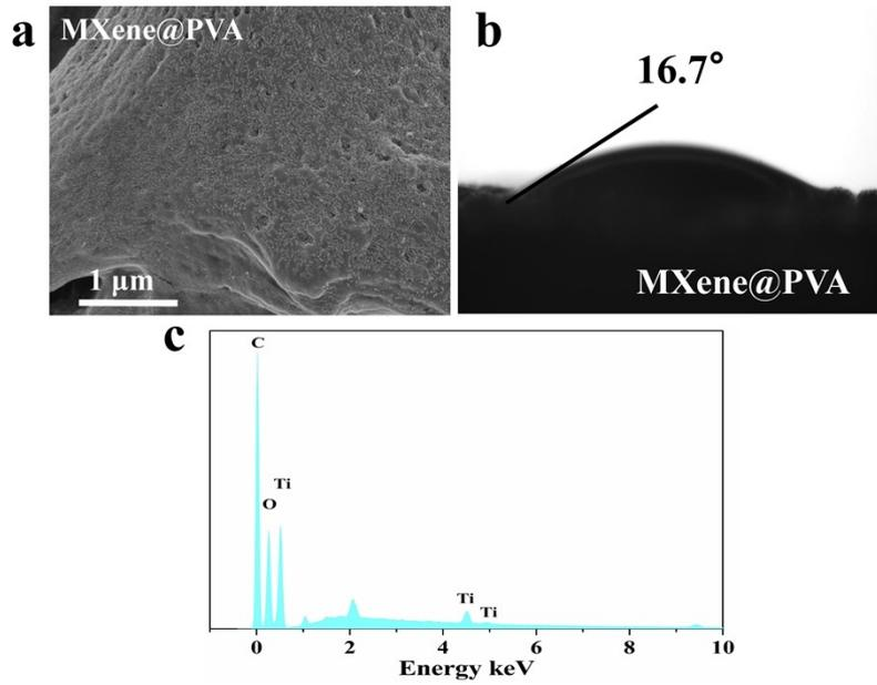
**Figure S3.** (a) SEM images of MXene@PVA (1 μm); (b) The contact angle measurement of MXene@PVA; (c) EDS spectrum of MXene@PVA hydrogel.
