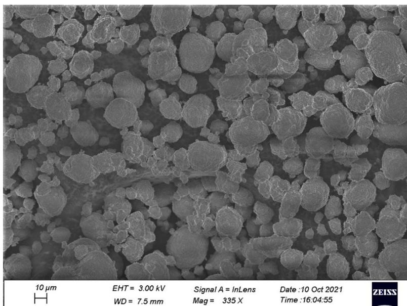
Figure S1. SEM image of commercial hydroxyapatite microparticles purchase from Sigma-Aldrich.
