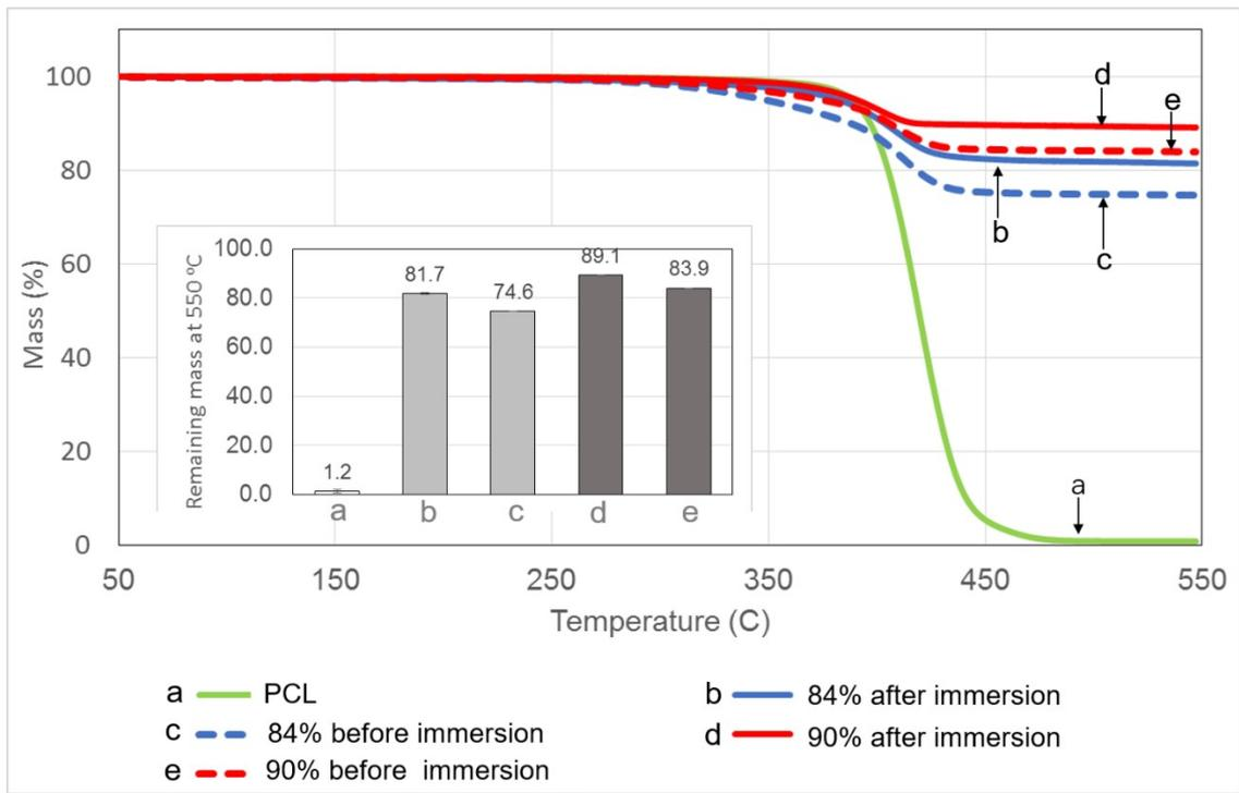
Figure S7. Measurement of hydroxyapatite content in scaffolds using thermogravimetric analysis. Inset shows the experimentally measured hydroxyapatite contents. Legends are the theoretical hydroxyapatite contents.
