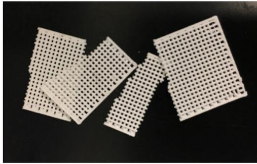
Figure S4. 3D printed PCL/HA sheet (4 layers) without PEG fractured easily after slight bending.
