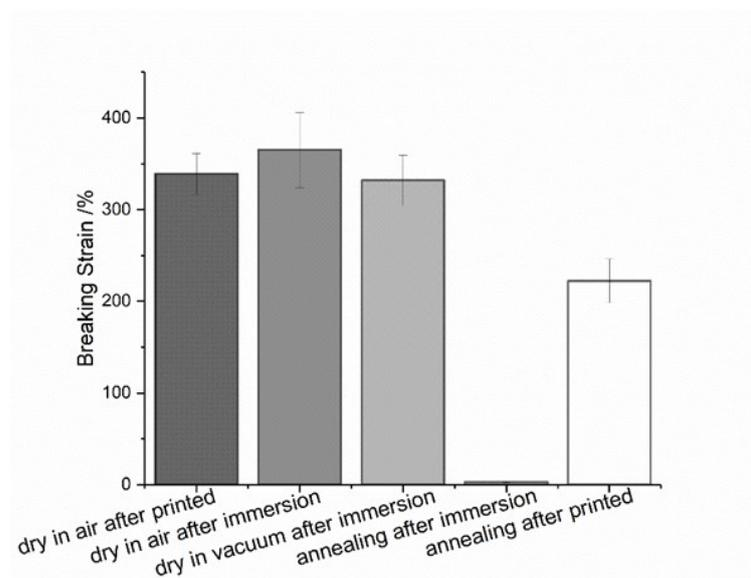
Figure S14. Breaking strain of PCL/PEG/HA struts with different treatments. Annealing (57°C) of struts after immersion in water removed ductility. Data represent mean  $\pm$  SD, n=5.
