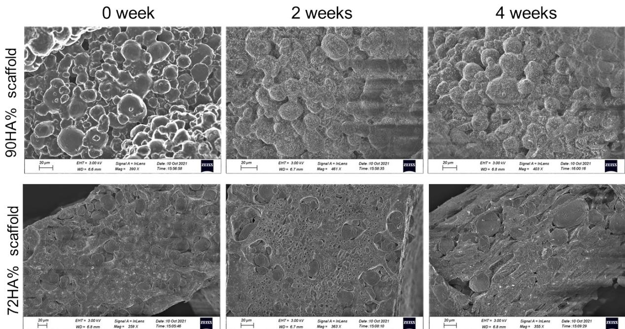
Figure S8. SEM images of scaffolds with two different hydroxyapatite contents after soaking in simulated body fluid for different times. The 90%HA scaffolds show white speckles which indicate the presence of precipitated minerals on the strut surface.
