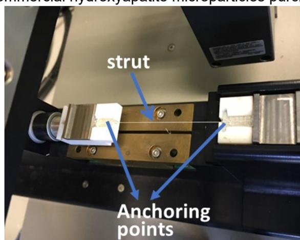
Figure S2. Tensile testing of a single strut.
