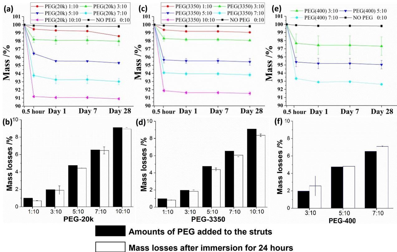
Figure S6. (a) Mass change of PCL/PEG/HA scaffolds (PCL:HA=1:9) after immersion in water. (b) Comparison of the theoretic amounts of PEG and measured amounts of leached PEG.
