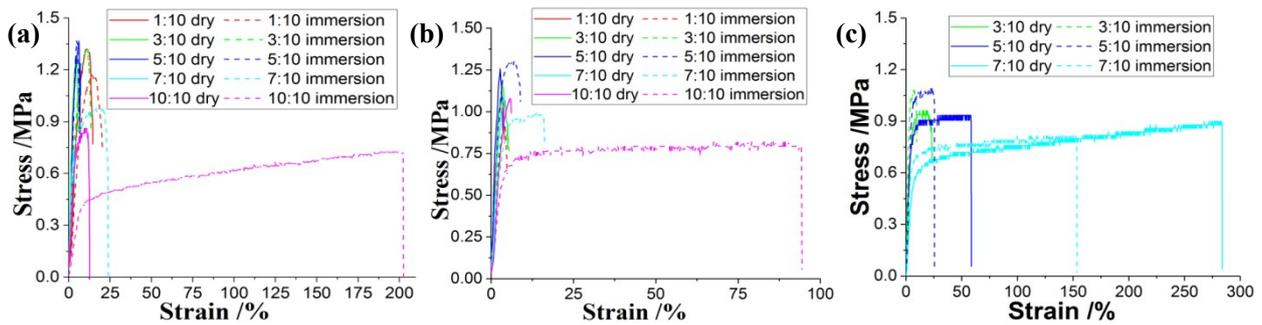
Figure S5. Representative tensile stress-strain curves of PEG/PCL/HA struts: (a) PEG(20k), (b) PEG(3350), and (c) PEG(400). The mass ratio of PCL to HA is fixed to 1:9. The mass ratio of PEG : PCL are 1:10, 3:10, 5:10, 7:10 and 10:10.
