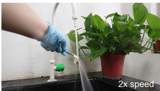
**Movie S3:** The  $P_{30}C_3T_3$  (MBAm<sub>0.6</sub>) hydrogel still adhered firmly to the surface of porcine skin after being washed by a high-pressure liquid.
