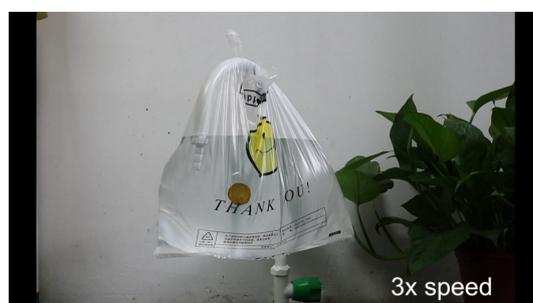
**Movie S4:** The sealing effect of the  $P_{30}C_3T_3$  (MBAm<sub>0.6</sub>) hydrogel on the water leakage by a blocking test.
