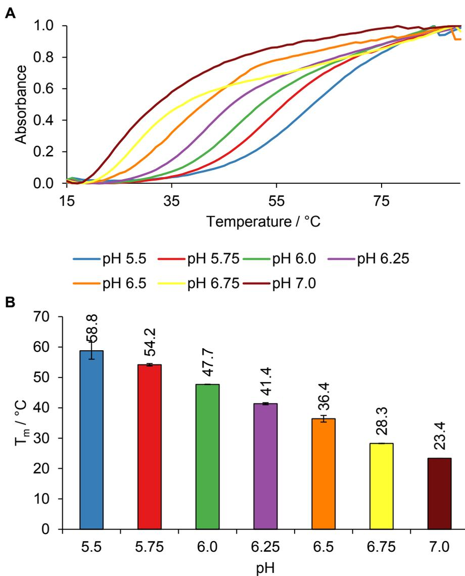
(A) Representative UV-melting curve of 1C; (B)  $T_m$  values of 1C ( $n = 2$ , error bars represent standard error).
