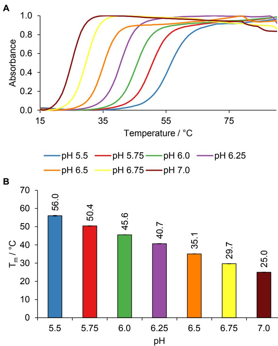
(A) Representative UV-melting curve of IM-CT; (B)  $T_m$  values of IM-CT ( $n = 2$ , error bars represent standard error).
