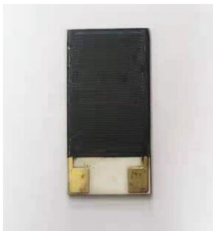
Fig. S6 Photograph of an interdigitated electrode with deposited SnS 2 /Pt 3 Sn for gas sensing.
