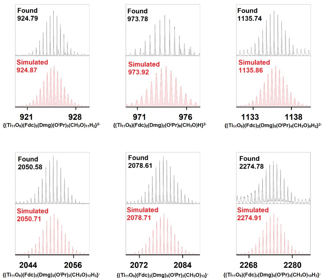
Figure S25. The isotope distributions of main peaks of ESI-MS spectrum of \{\text{Ti}_{11}\text{Fc}_2\} .
