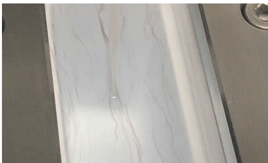
Figure 3. Photograph of a peptoid-AuNP composite monolayer at the air-water interface after compression in a Langmuir trough, revealing surface features that are perpendicular to the force of the compression.
