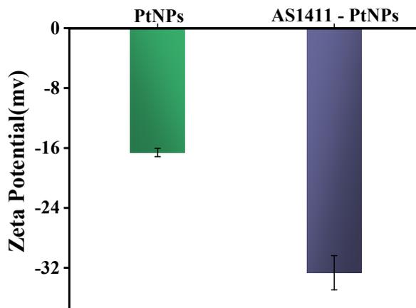
**Fig. S3** Potential characterization of AS1411 functionalization of PtNPs. Almost twice the potential increase indicated effective modification of thiolated AS1411 aptamer on the surface of PtNPs.
