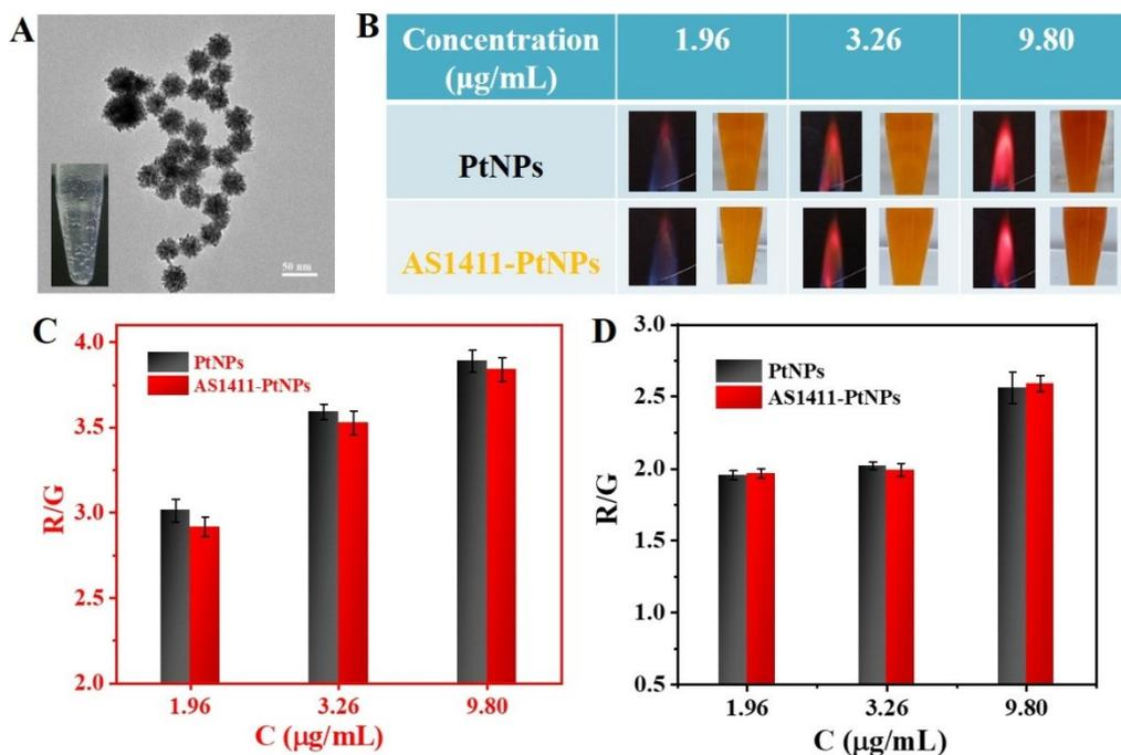
**Fig. S2** (A) TEM image of PtNPs. The inset showed the catalytic reaction of  $\text{H}_2\text{O}_2$  by PtNPs. (B) The effect of aptamer modification on the catalytic activity of PtNPs. Comparison of the catalytic activity between PtNPs and AS1411-PtNPs using the detection mode of (C) atomic flame and (D) molecular colorimetry, respectively.
