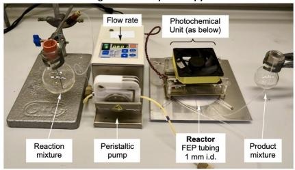
Light source:  $6 \times 1.7W$  UVA (365 nm) LEDs. Reactor: Spiral wound FEP tubing with 6 mL capacity. **SAFETY NOTE**: In operation, the photochemical unit is housed within a protective cover.
