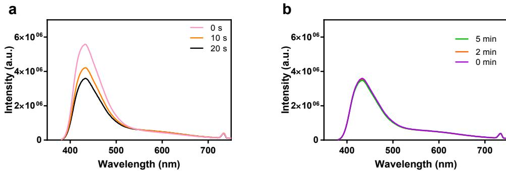
**Figure S6.** a) Photoluminescence spectra of polymer **C8** under continuous 365 nm excitation for several time. b) Photoluminescence spectra of polymer **C8** at certain time points post UV irradiation.
