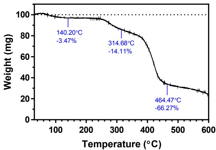
**Figure S12.** Thermogravimetric analysis of polymer C8.
