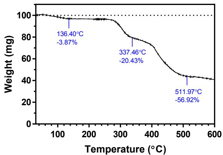
**Figure S13.** Thermogravimetric analysis of polymer **C9**.
