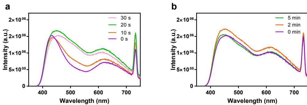
**Figure S5.** a) Photoluminescence spectra of polymer **C7** under continuous 365 nm excitation for several time. b) Photoluminescence spectra of polymer **C7** at certain time points post UV irradiation.
