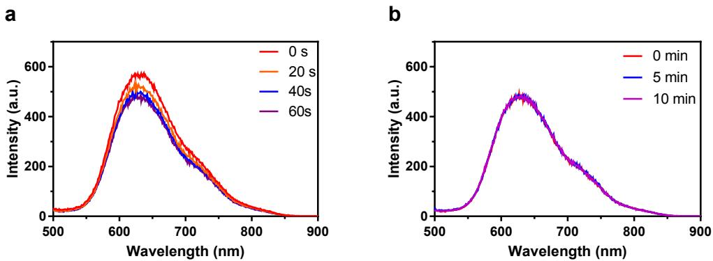
**Figure S4.** a) RTP spectra of polymer **C8** under continuous 365 nm UV irradiation for certain time. b) RTP spectra of polymer **C8** in dark at various time points post 365 nm UV irradiation.
