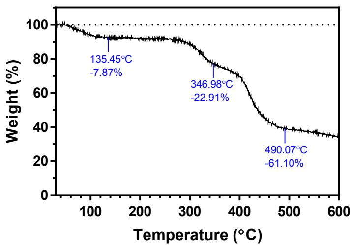
**Figure S11.** Thermogravimetric analysis of polymer C7.
