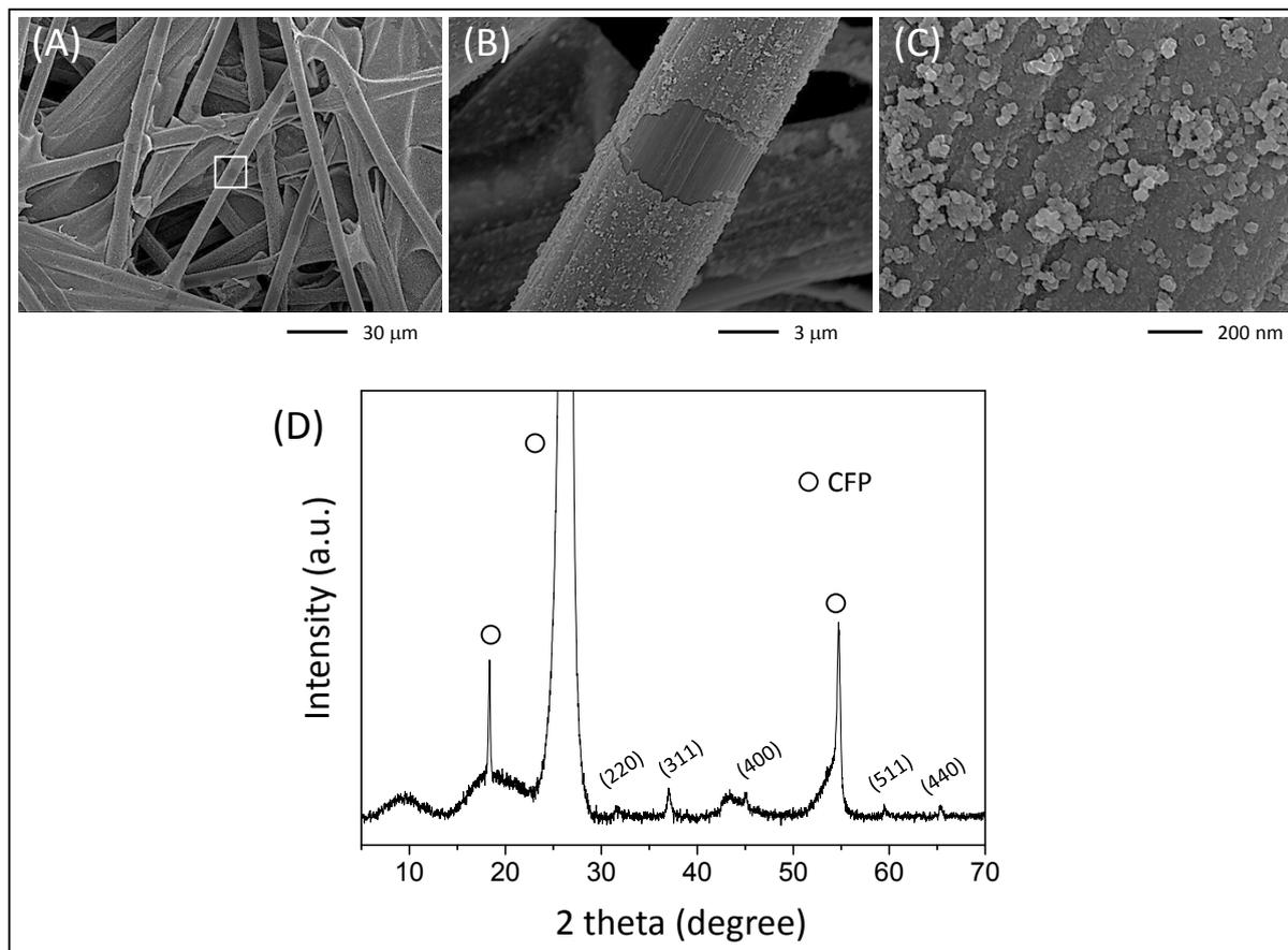
**Figure S12.** SEM images (A-C) and XRD pattern (D) of MnCo<sub>3</sub>O<sub>4</sub>(0.01)/CFP electrode after durability test for 10,000s. The white boxes in (A) is enlarged in (B).
