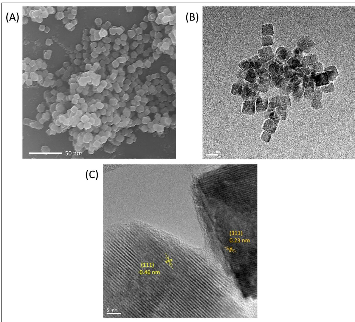
**Figure S5.** SEM (A), TEM (B), and HRTEM (C) images of collected nanocubes from the colloidal of the MnCoO film.
