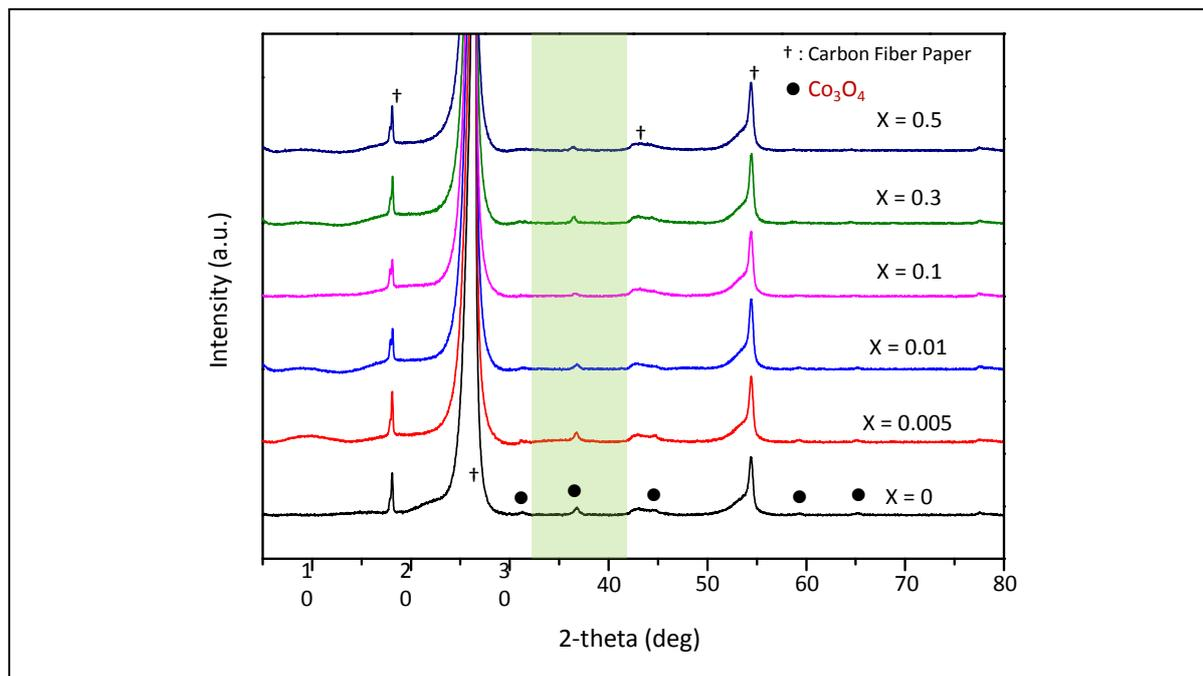
**Figure S7.** XRD data of Mn<sub>x</sub>Co<sub>3-x</sub>O<sub>4</sub> thin film on CFP substrate.
