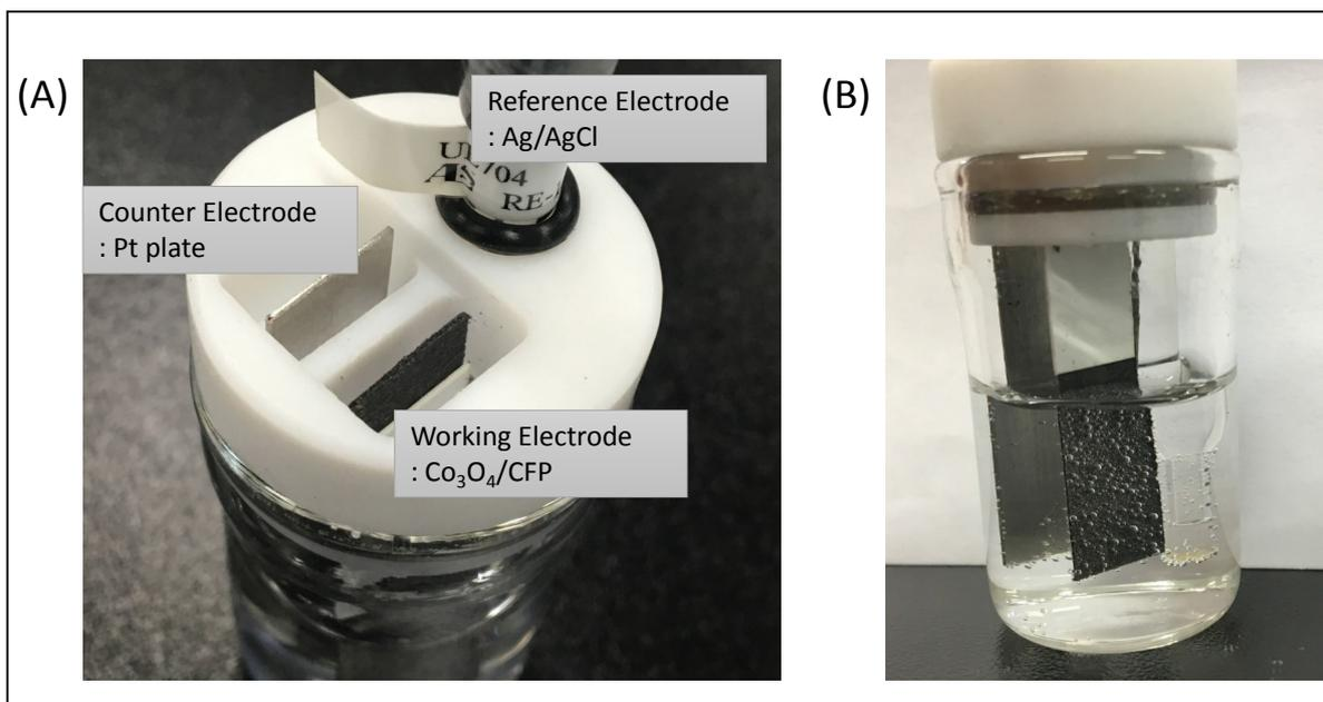
**Figure S10.** Top and side views of the electrode arrangement for OER measurement.
