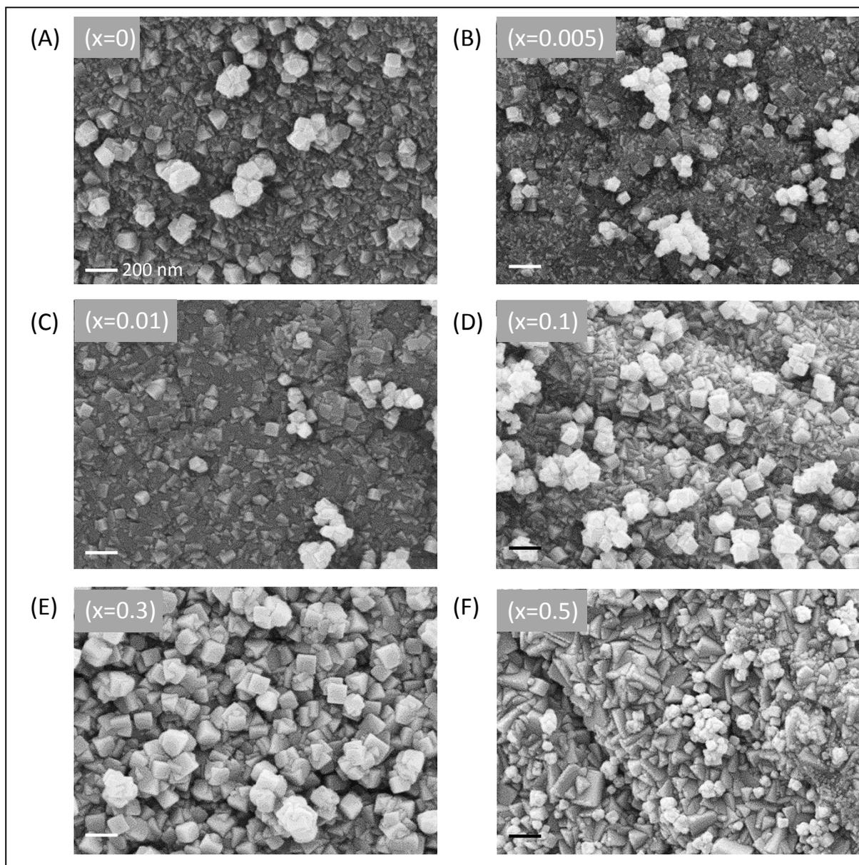
**Figure S9.** SEM images of the  $\text{Mn}_x\text{Co}_{3-x}\text{O}_4$  thin film on CFP substrate.
