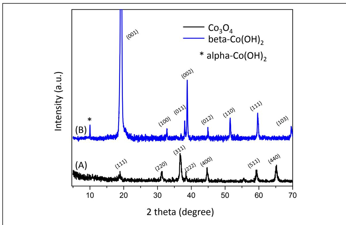
**Figure S6.** XRD patterns for the powdery  $\text{Co}_3\text{O}_4$  nanoparticle samples obtained by the topotactic method and for the  $\text{Co(OH)}_2$  obtained by the conventional hydrothermal method. The asterisk in (B) indicates the alpha phase of  $\text{Co(OH)}_2$ .
