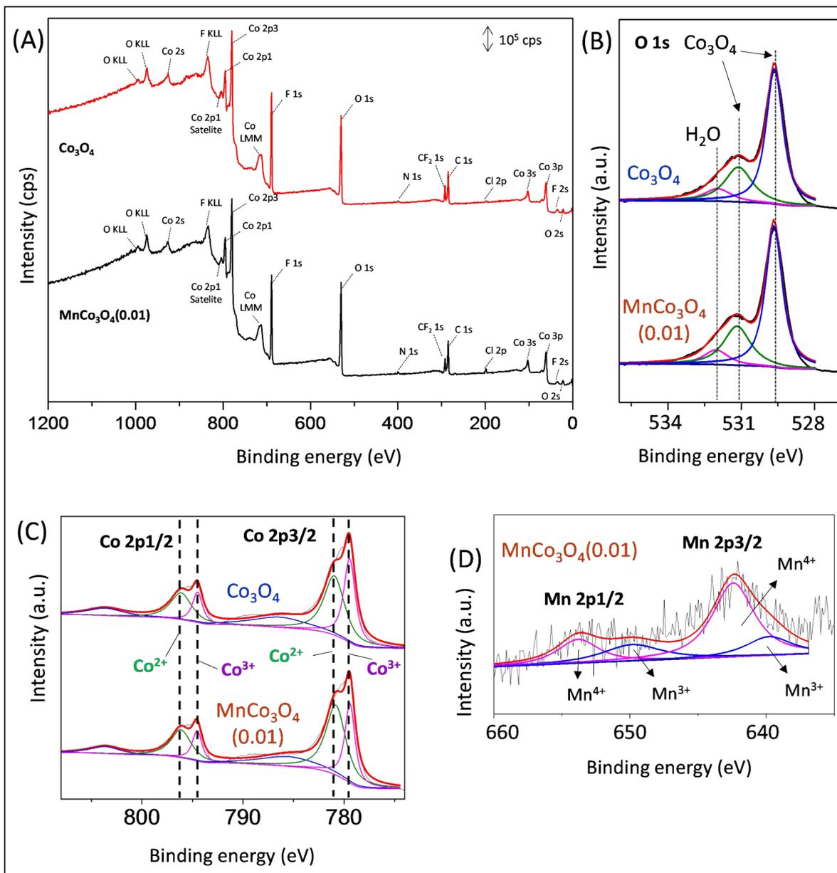
**Figure S8.** (A) XPS wide spectra of  $\text{Co}_3\text{O}_4$ /CFP (top) and  $\text{MnCo}_3\text{O}_4(0.01)$ /CFP (bottom). (B) O 1s and (C) Co 2p core-level XPS spectra of  $\text{Co}_3\text{O}_4$ /CFP and  $\text{MnCo}_3\text{O}_4(0.01)$ /CFP. (D) Mn 2p core-level XPS spectrum of  $\text{MnCo}_3\text{O}_4(0.01)$ /CFP.
