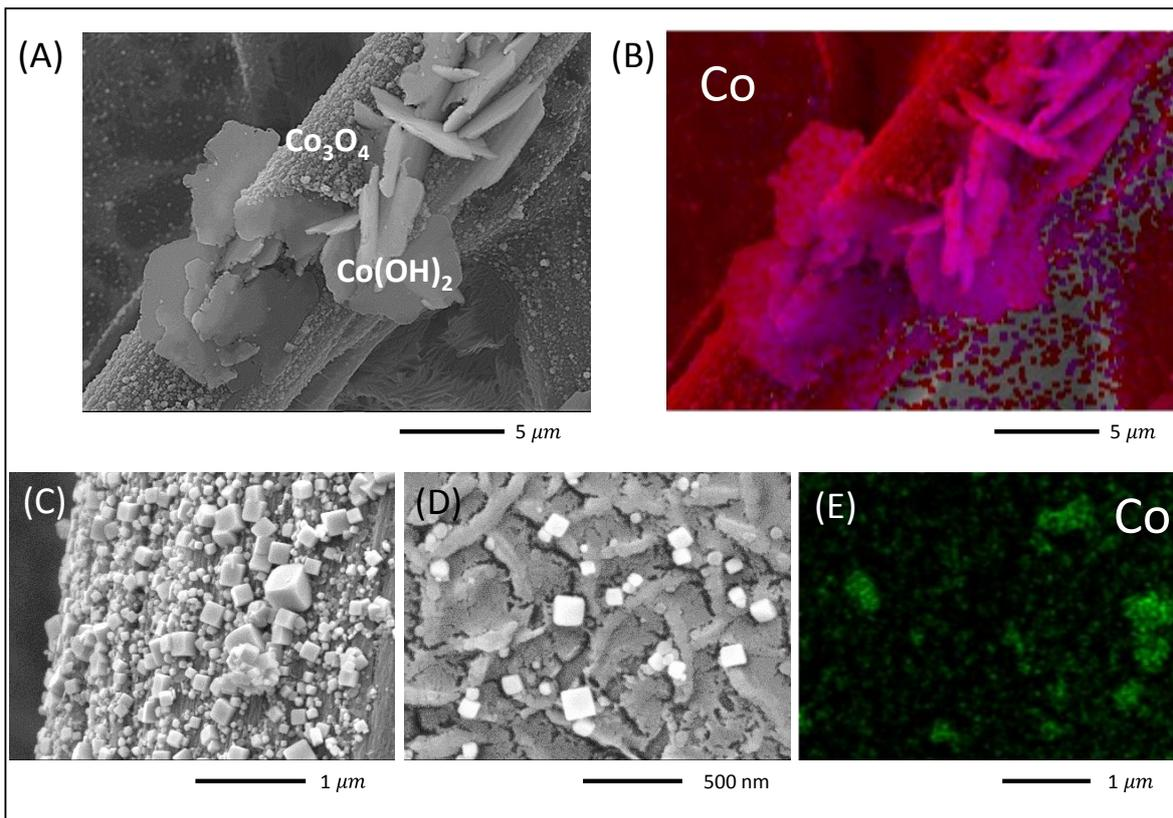
**Figure S1.** (A, C, D) SEM images and (B, E) elemental map (Co) of  $\text{Co}_3\text{O}_4/\text{CFP}$  prepared by the hydrothermal method.
