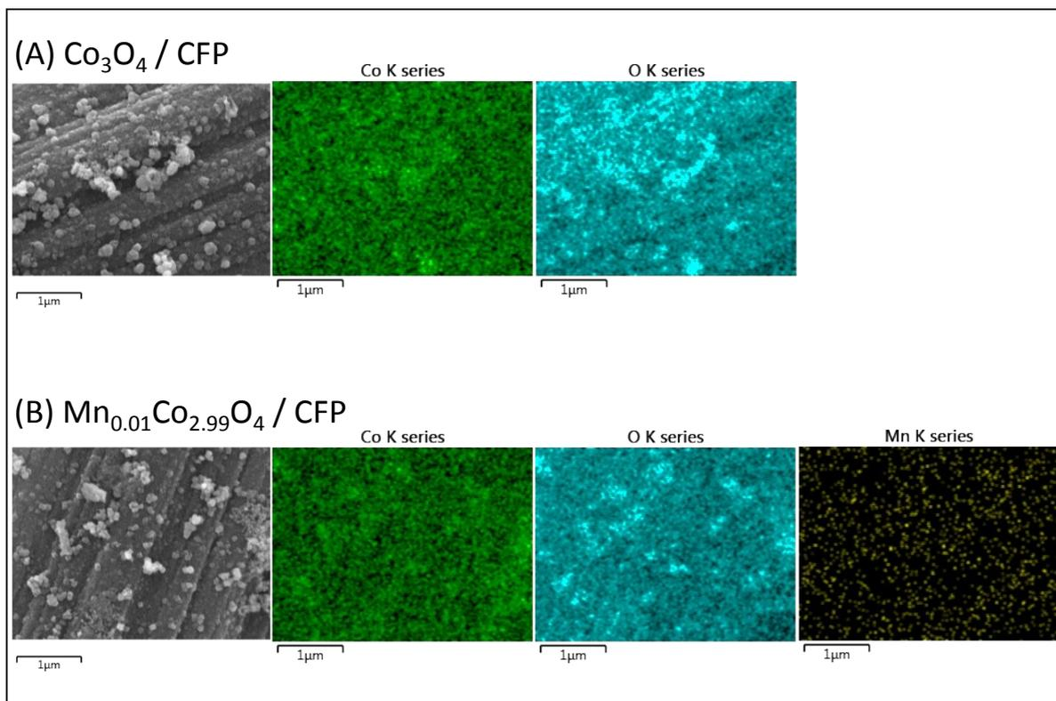
**Figure S3.** SEM images and elemental maps of (A)  $\text{Co}_3\text{O}_4$ /CFP and (B)  $\text{MnCo}_3\text{O}_4(0.01)$ /CFP films.
