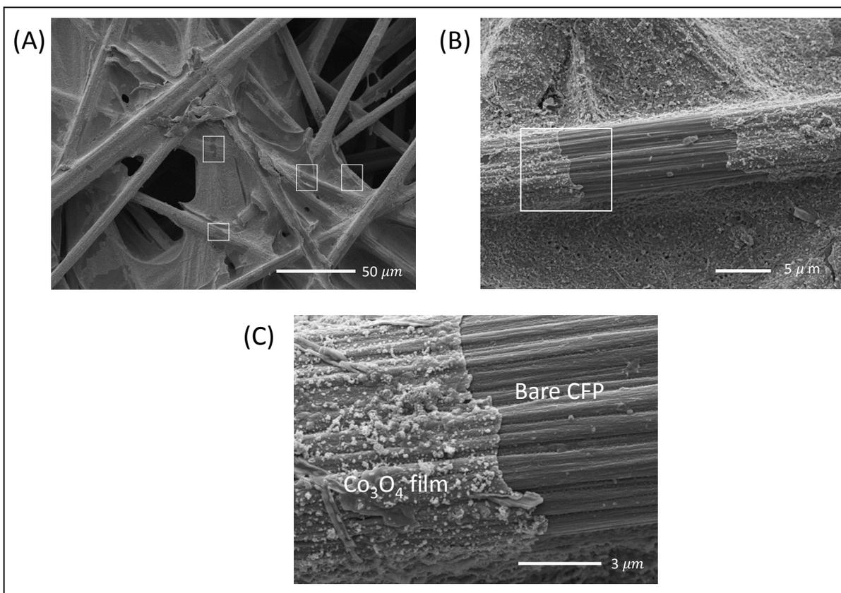
**Figure S2.** SEM images of  $\text{Co}_3\text{O}_4/\text{CFP}$  prepared by the topotactic method. (C) An enlarged image of the area in the white box shown in (B). The white boxes in (A) indicate the areas not covered by the  $\text{Co}_3\text{O}_4$  thin film.
