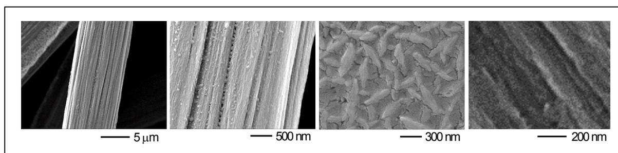
**Figure S4.** SEM images of bare CFP substrate.
