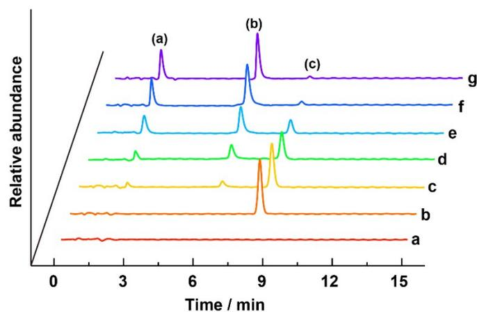
Figure S15. HPLC kinetic profiles of PA molecules (5 mM) reacting with 5 mg mL<sup>-1</sup> MAO-A. a) Blank; b) PA molecules; c–g) the reaction between PA molecules and MAO-A for 6, 12, 18, 24, 30 min, respectively.
