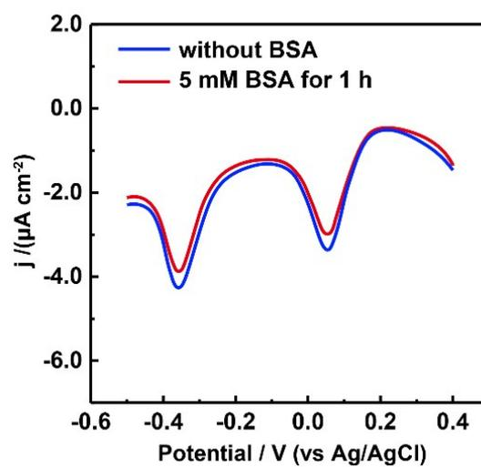
**Figure S23.** DPVs obtained at CFME/Au/MB+PA electrode in aCSF solution without BSA and with 5 mM BSA for 1 h.
