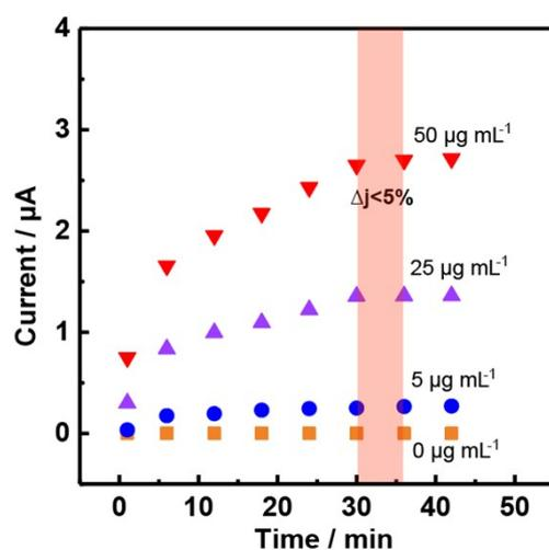
**Figure S20.** Time-dependent peak current obtained by CVs at CFME/Au/MB+PA electrode in aCSF solution (pH 7.4) in the presence of 0, 5, 25, 50  $\mu\text{g mL}^{-1}$  MAO-A.
