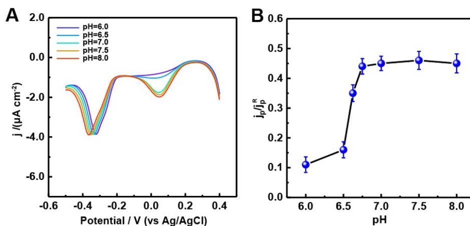
**Figure S25.** The obtained DPVs (A) and  $j_p/j_p^R$  values (B) after CFME/Au/MB+PA electrode was immersed into aCSF solution with pH range from 6.0 to 8.0 for 30 min.
