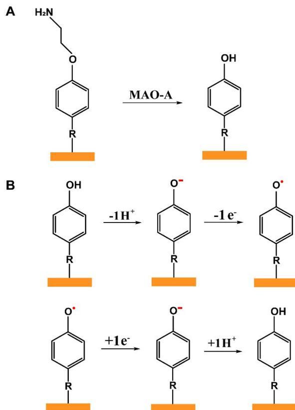
**Figure S19.** (A) Chemical process (A) and electrochemical redox process (B) occurred on CFME/Au/MB+PA electrode in MAO-A containing aCSF solution (pH 7.4).
