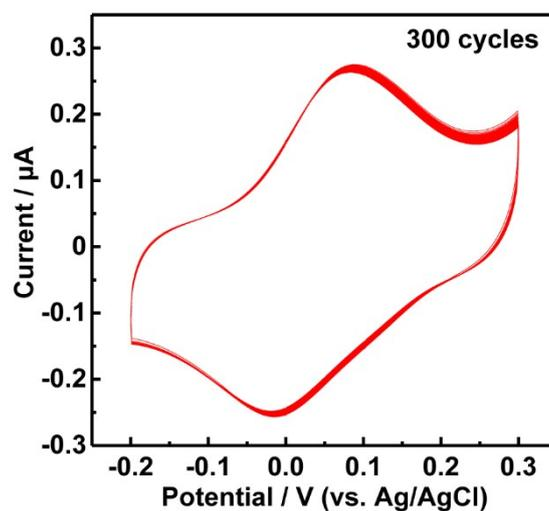
**Figure S21.** CVs obtained at GCE/Au/MB+PA electrode for 300 cycles in aCSF solution (pH 7.4) containing 4  $\text{mU mL}^{-1}$  MAO-A.
