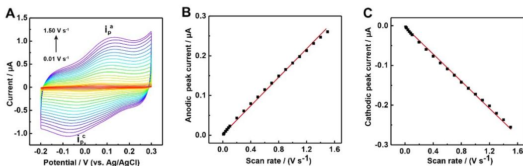
**Figure S24.** (A) CVs obtained at GCE/Au/MB+PA electrode at the scan rates of 10, 20, 40, 60, 80, 100, 200, 300, 400, 500, 600, 700, 800, 900, 1000, 1100, 1200, 1300, 1400 and 1500  $\text{mV s}^{-1}$  (from inner to outer) in aCSF solution (pH 7.4) containing 4  $\text{mM mL}^{-1}$  MAO-A, (B) Plots of anodic peak current versus scan rate, (C) Plots of cathodic peak current versus scan rate.
