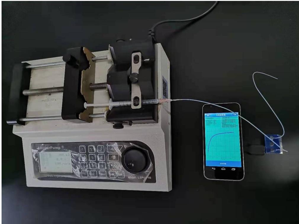
Fig. S3 The microfluidic biochip and smartphone-based detection system for CR.
