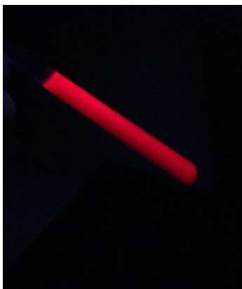
Figure S1. Picture of rac - 2.H(PF 6 ) 2 at 77 K in MeTHF irradiated at 254nm.
